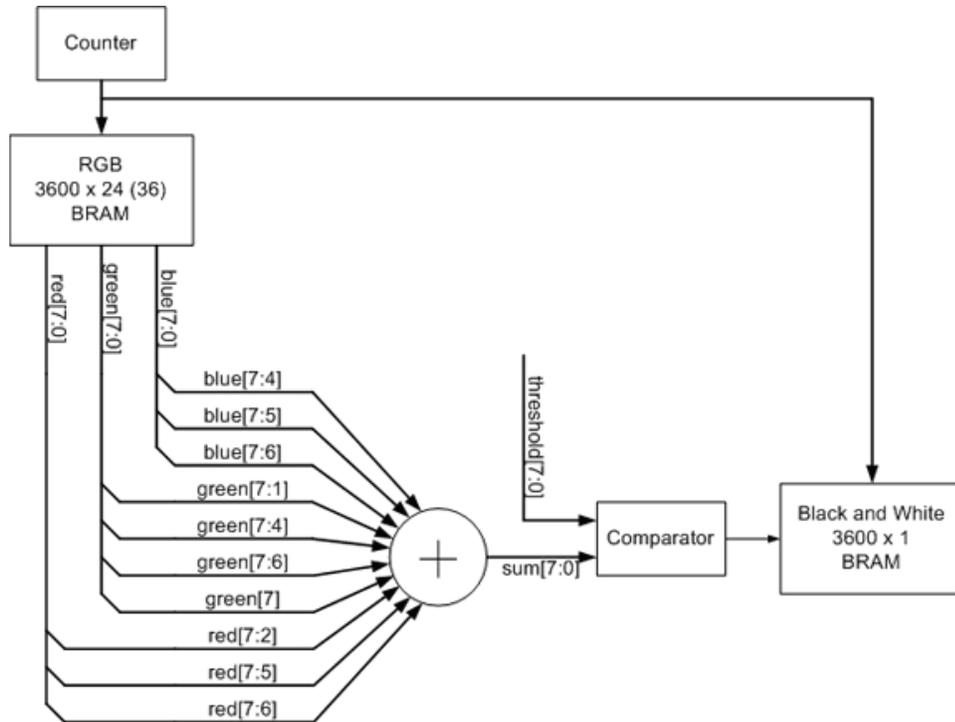
Figure 5.24: RGB to black and white conversion circuit
