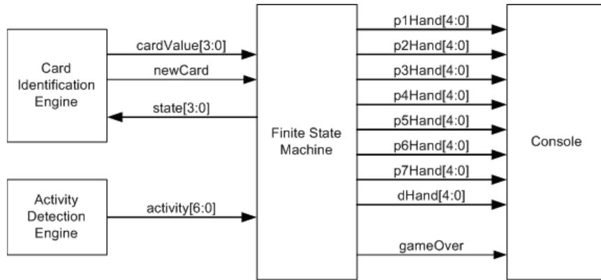
Figure 5.16: Finite State Machine Signals
