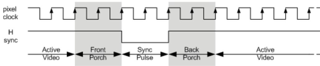
Figure 5.10: Horizontal Synchronization
