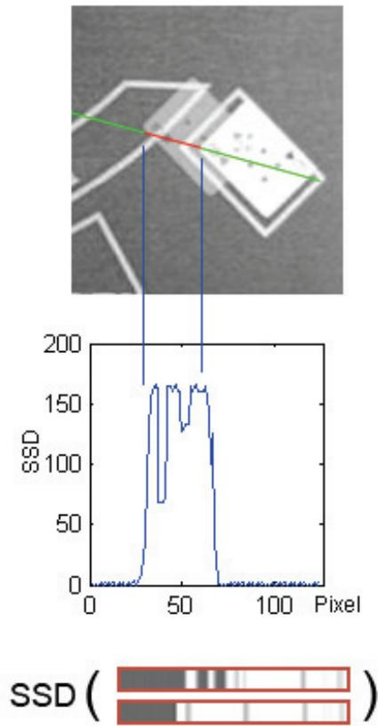
Figure 5.20: Correlation between detection lines and SSD values
