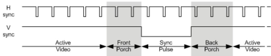
Figure 5.11: Vertical Synchronization
