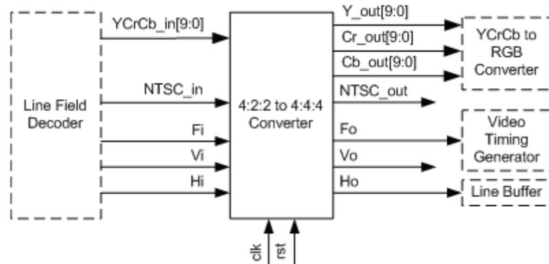
Figure 5.7: 4:2:2 to 4:4:4 Converter Block Diagram
