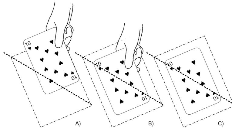
Figure 4.7: Dealer's hand not perceived by detection line
