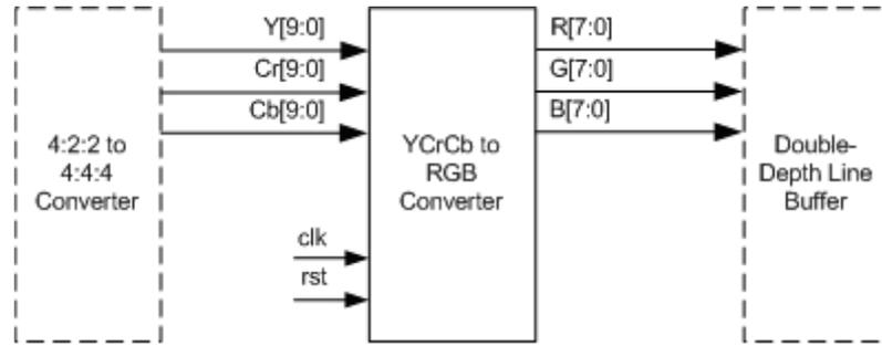
Figure 5.9: YCrCb to RGB Converter Block Diagram
