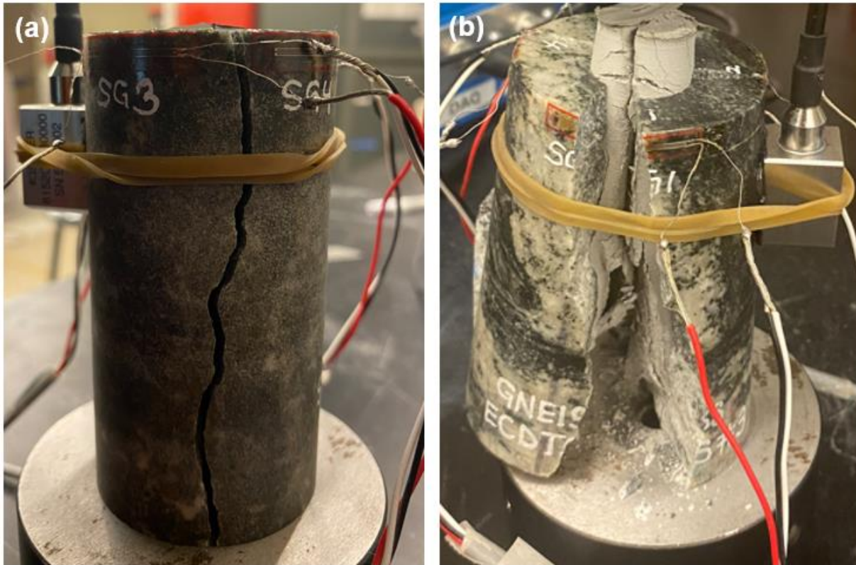
Figure 5.5 Specimen Failure Pattern. (a) Sudbury Breccia Specimen. (b) Intermediate Gneiss Specimen.
