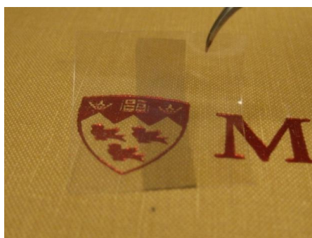
Figure 4.6 a) PDMS stamping of films on PET b) a single strip of nanotubes on PET [5]
