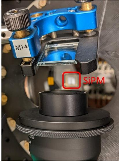
(a) A mirror reflects the beam onto the SiPM located inside the ETS cryostat, which permits testing at cryogenic temperatures. A single SiPM is visible inside the chamber.
