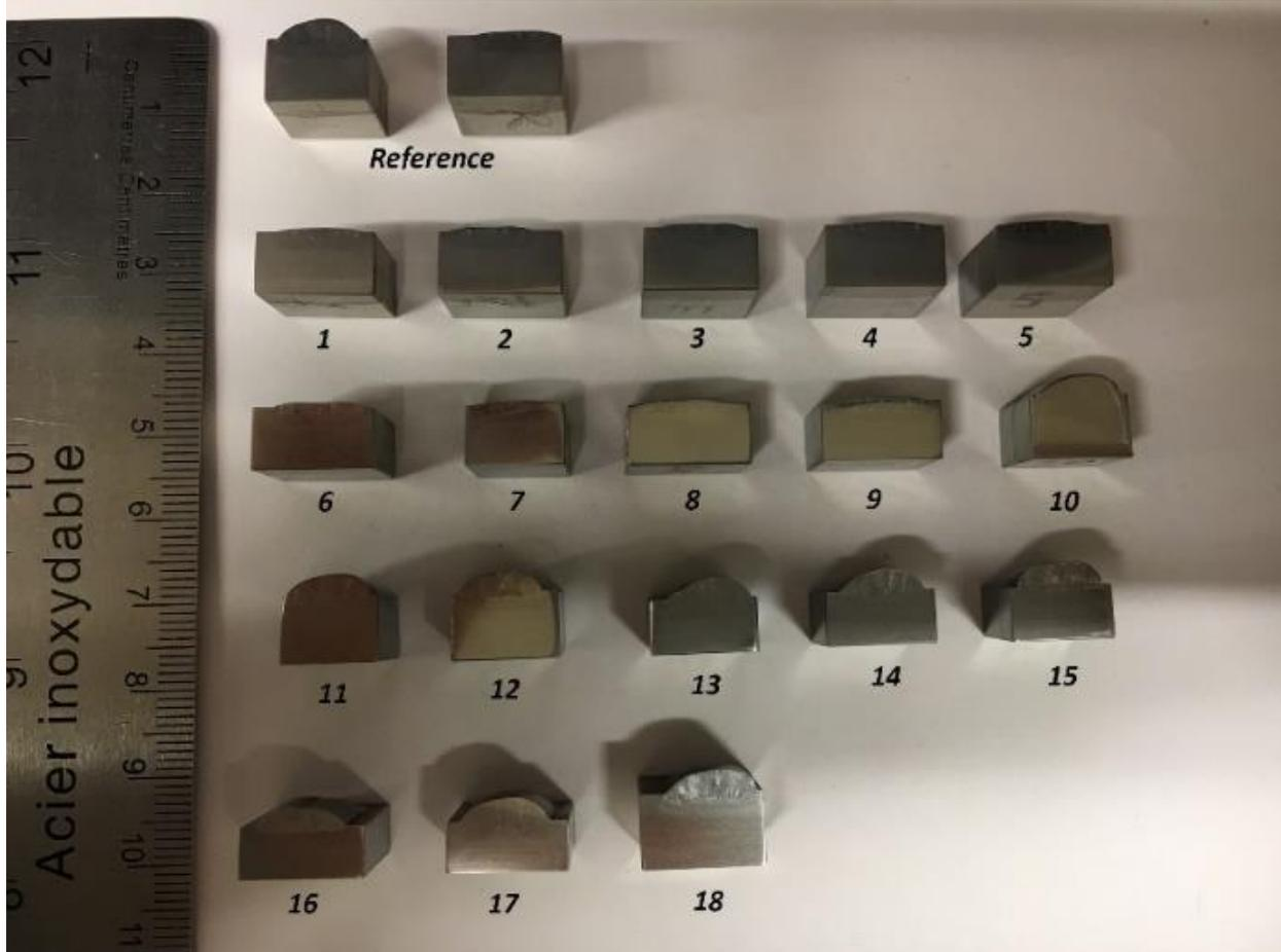
Figure 4-6 Specimens fabricated via wire DED process under the Taguchi experiment design for Y-Z plane data collection.
