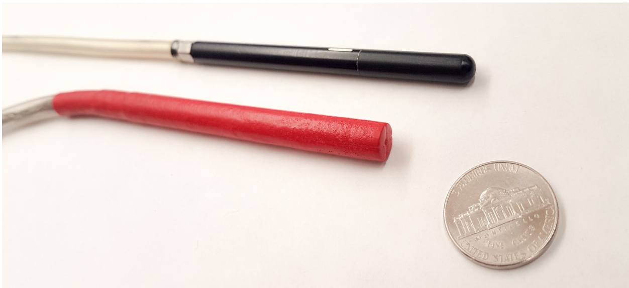
Figure 6.1. Photograph of a side-by-side comparison of Aerrow MK7 (red), an Exradin A1SL ionization chamber (black), and a coin for size reference. The ionization chamber pictured is the same one used for comparing the dosimetric performance of Aerrow MK7 in quasi-adiabatic mode. The red and porous external appearance of Aerrow MK7 is given by the waterproof plastic coating that surrounds the entire acrylic stem and part of the cable.
