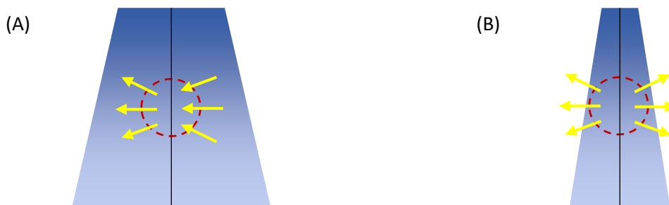
Figure 3.1. A schematic depiction of (A) LCPE in a broad photon field and (B) loss of LCPE in a narrow photon field. In (A), external secondary electrons (yellow) enter laterally into the central axis region (red) and compensate for the secondary electrons exiting the central axis region, but there is no such compensation in (B).
