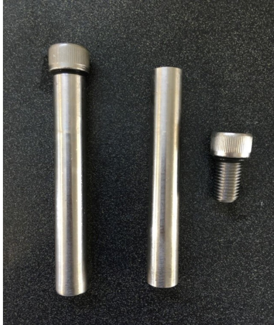
Figure 3.1 The stainless steel capped test tube used for oil bath
