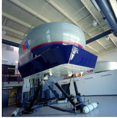
Figure 2.1: Flight simulator's 6-degree of freedom hydraulics[Courtesy United Virtual]
