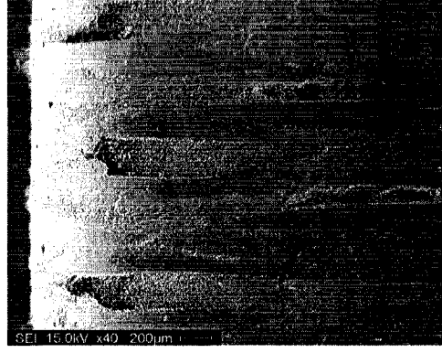
Figure 1.11: SEM Image Showing Fiber Pull Out Obtained at N = 5,000 rpm and f = 20 mm/rev During Drilling of Woven Graphite Epoxy Composite with a Standard Point Carbide Drill.
