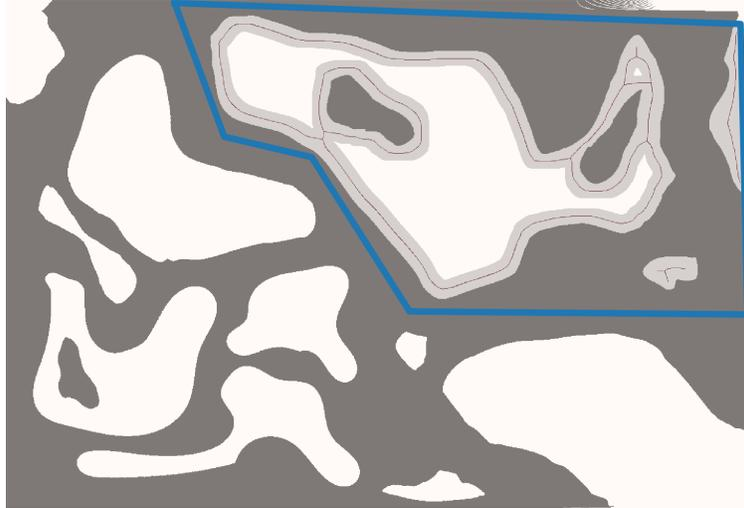
**Figure 3.3:** An illustration of free space segmentation and skeletonization. The blue polygon indicates the region of interest in which we require full coverage. The white area and bright gray area represent the wide and narrow space respectively and the red curve is the generated skeleton.
