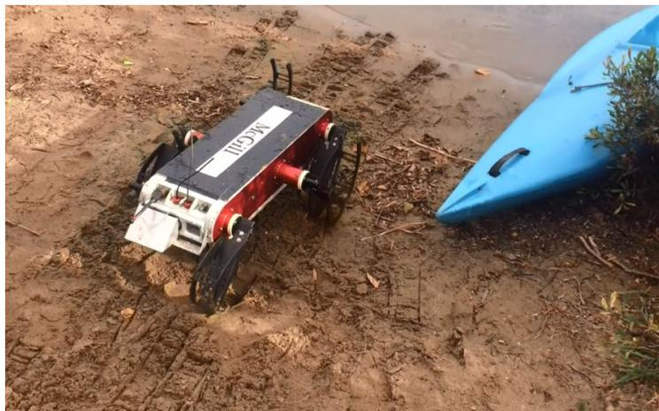
**Figure 3.4:** The amphibious Aqua robot walking on the shoreline.
