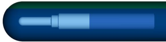
Figure 2.3: Exradin A12 at 1 cm depth with an air/water XCSE shell.
