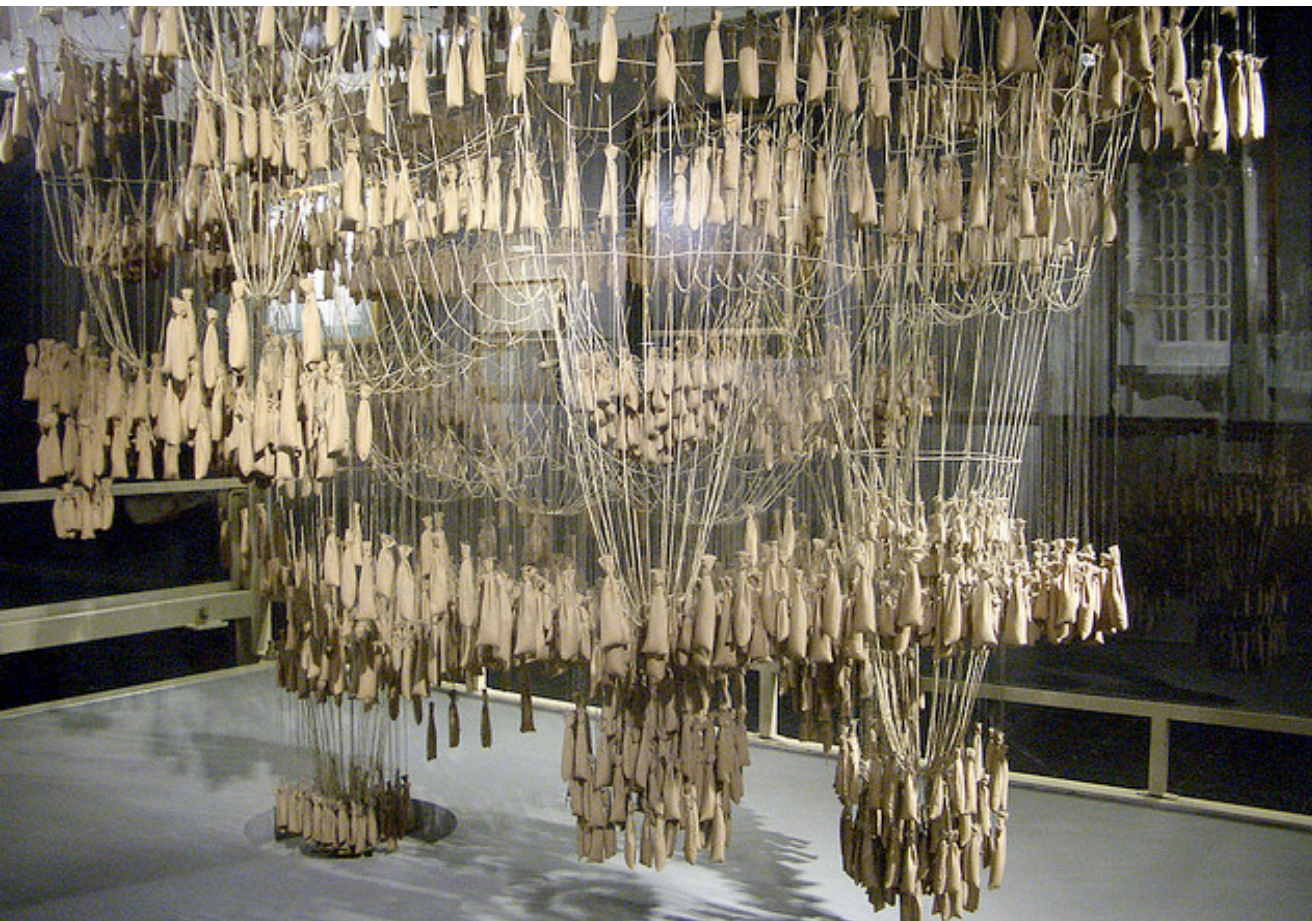
fig. 4 Reconstruction of Gaudí's hanging model (Tomlow, 1989)
