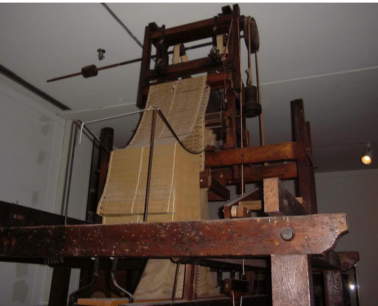
fig. 3 Jacquard loom with punch cards ca. 1840, from Smithsonian NMAH
