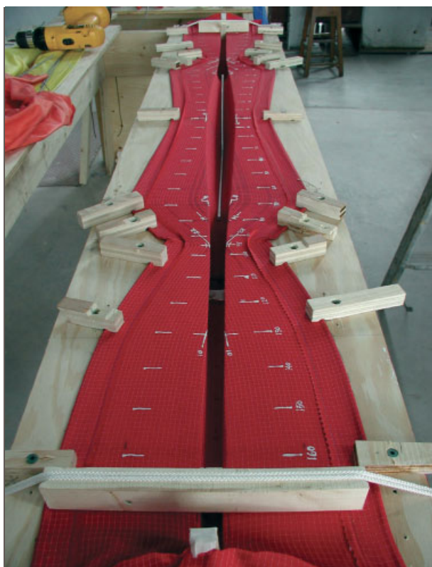
fig. 5 Beam model formwork and full-scale fabric formwork beam cast, Mark West, 2003
