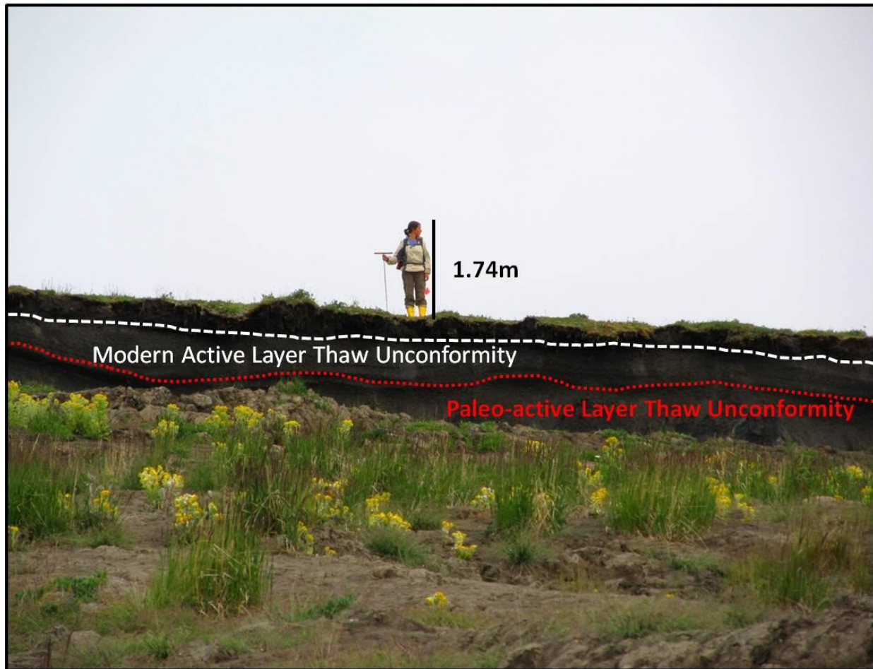
Fig. 3. 4.: Headwall view within the undisturbed section of Slump A , with lines demarcating the modern and paleo –active layer thaw unconformities.
