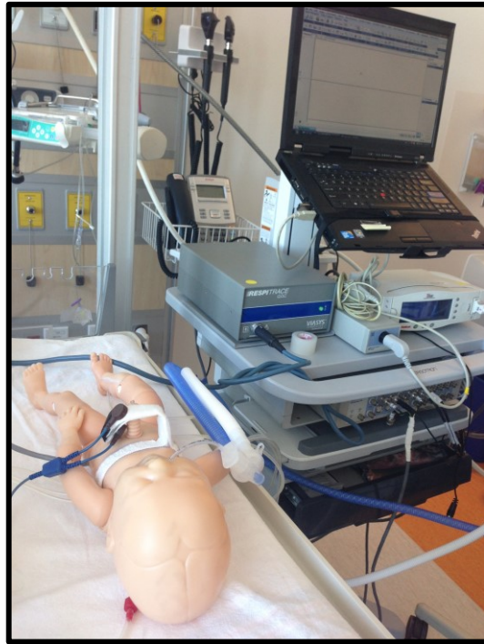
Figure A1. RIP band validation experimental set-up, showing the ventilated manikin, the SleepSense band placed around the chest of the manikin, and the data acquisition cart.
