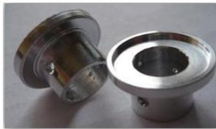
Figure 4.7: Custom-made aluminium coupler and its dimensions.
