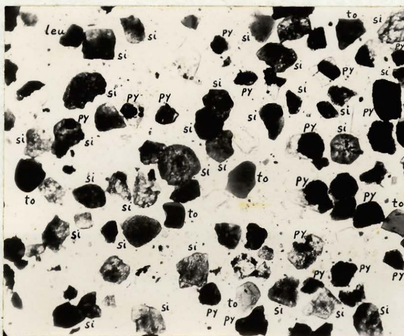
Fig. 2 - HM No.32, X69, plane polarized light. leu-leucoxene, py-pyrite, si-Siderite, to-tourmaline.
