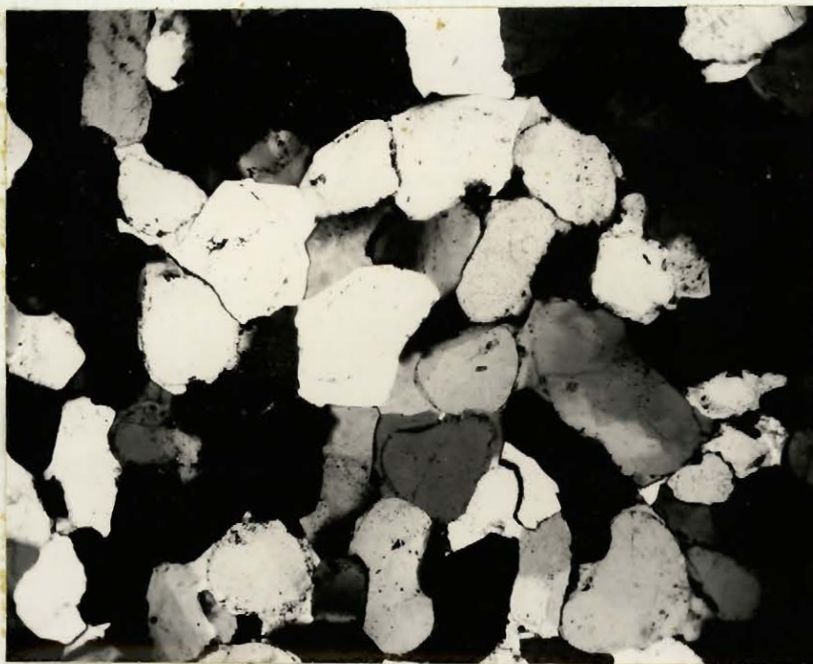
Fig. 2, T.S. No. 6, x60, as above, crossed nicols. Note angularity of grains due to secondary growths in optical continuity with detrital core.
