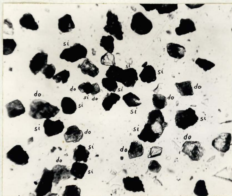
Fig. 1 - HM No.26, X68, plane polarized light. do-dolomite, si-siderite.
