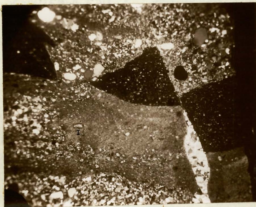
Fig. 2 - Shale, Shaly Sandstone : T.S.No.23, x 16, crossed nicols. Small movement along joint on right side with a calcite veinlet formed along the jointing plane. Shale band has been partially eroded, top centre and left. Visible grains mainly quartz. I - Area of lighter colour with pyrite around periphery.
