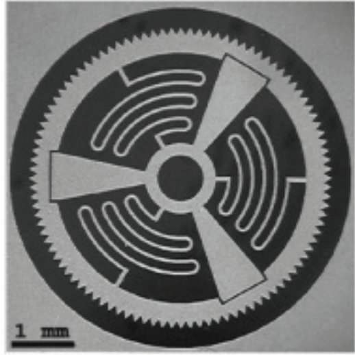
Figure 2–11: Optical image of a 5 mm diameter wheel made out of SU8 nanocomposite [60].
