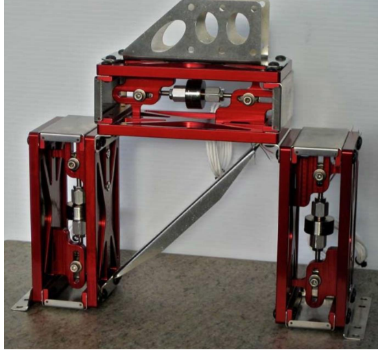
Figure 3–8: Kineoptics WTB 3.0 wind tunnel balance.
