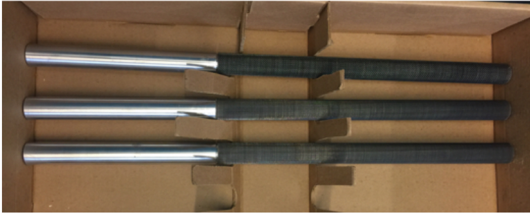
(a) Some cylinders with porous outer layer
