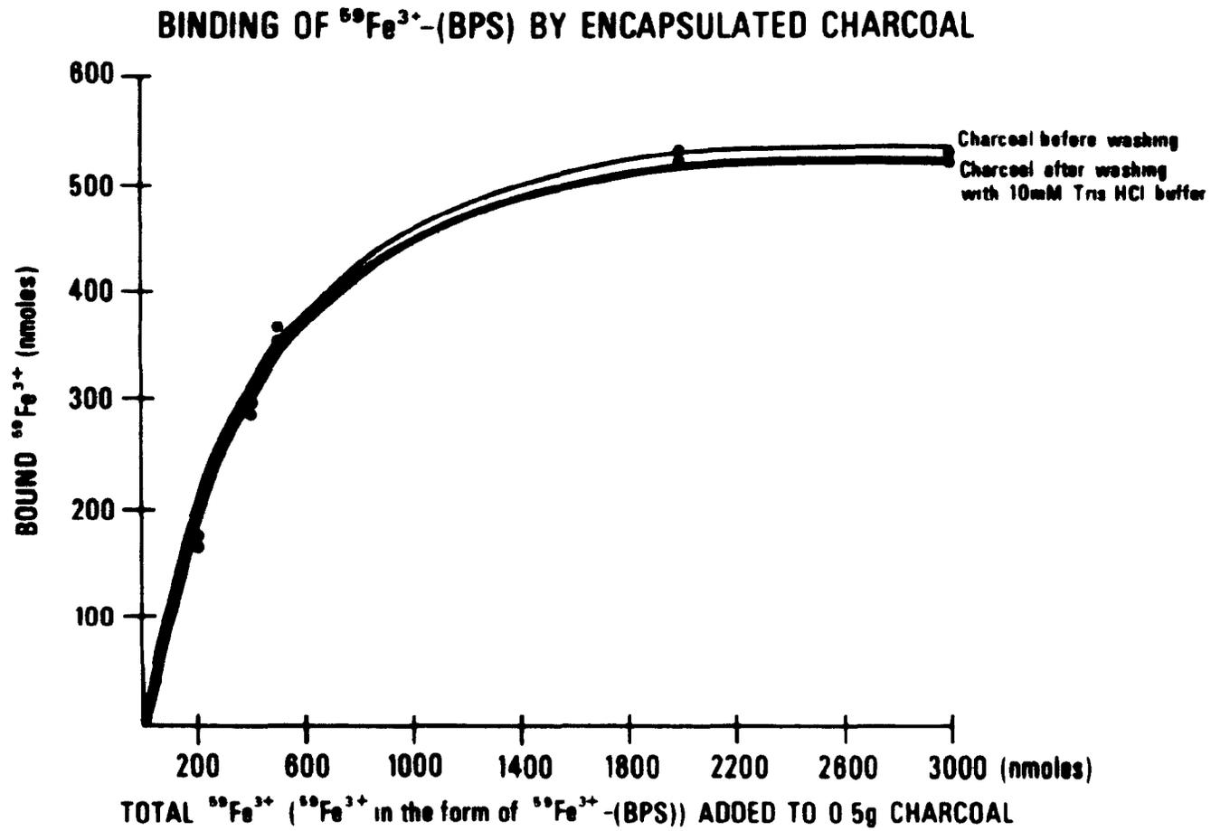
Iron-binding capacity of encapsulated activated charcoal.
