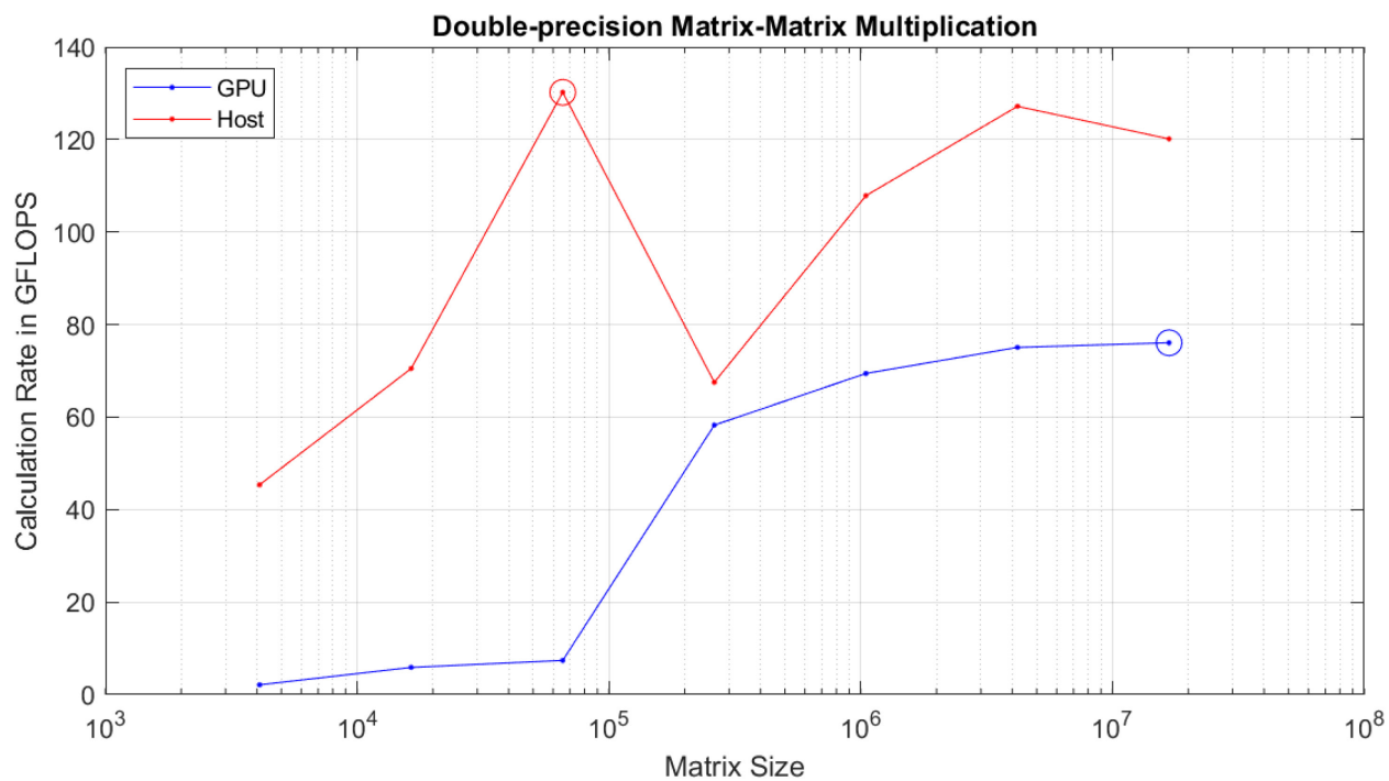
Figure 5.18: Rate of Matrix Multiplication Operation on i7-4710HQ and GTX 970M.
