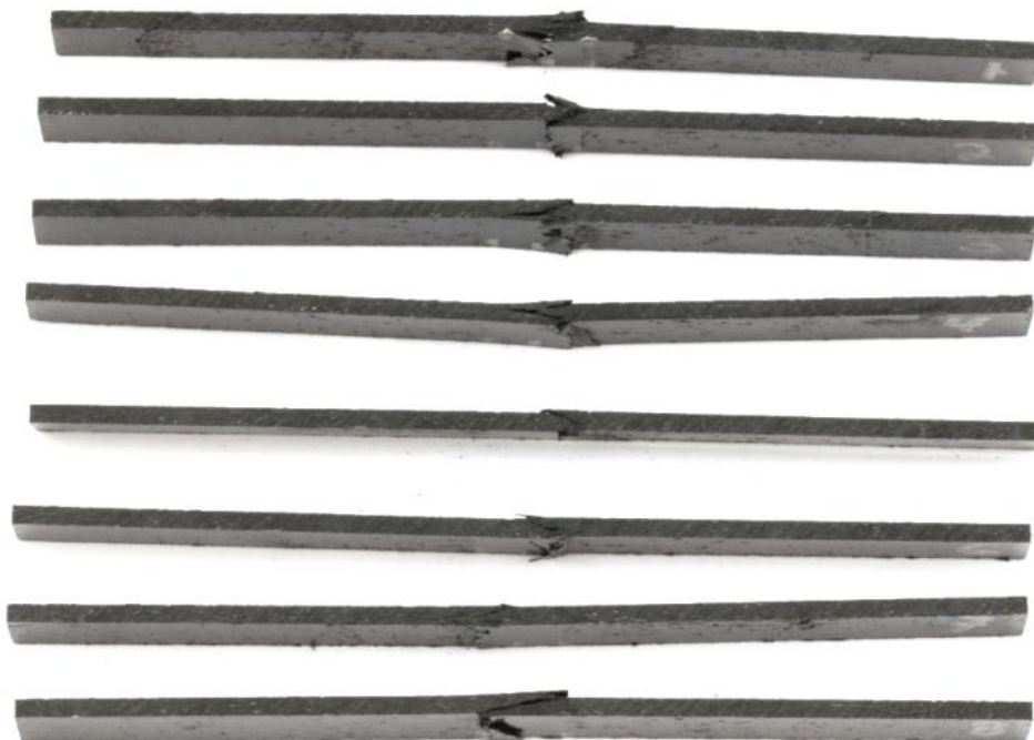
Figure E-5. M40 D6641-14 Compression specimens 1-9 (top-bottom).
