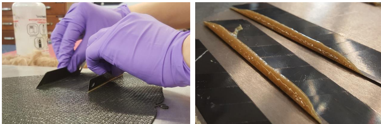
Figure 4-3. A razor blade being drawn across the hot prepreg surface (left) and some of the corresponding resin obtained cooling on a steel plate (right).
