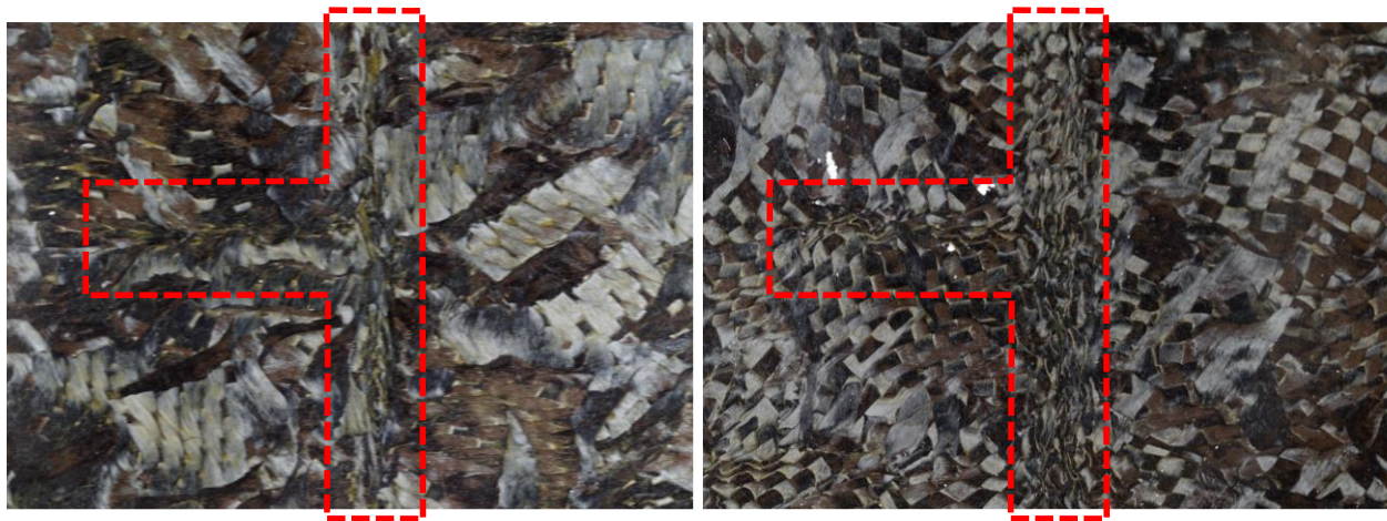
Figure 7-13. Print-through artifacts caused by the flow of fibre into the two rib features of a compound T-bracket: 8HS-strand part on the left and PW-strand part on the right.
