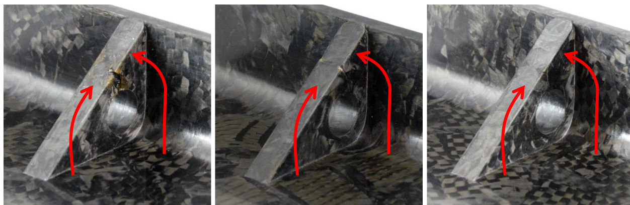
Figure 7-14. Close-up images of compound T-bracket secondary ribs showing the possible formation of a knit line. From left to right: PW strands moulded at 6 MPa; 8HS strands moulded at 6 MPa; PW strands moulded at 9 MPa.
