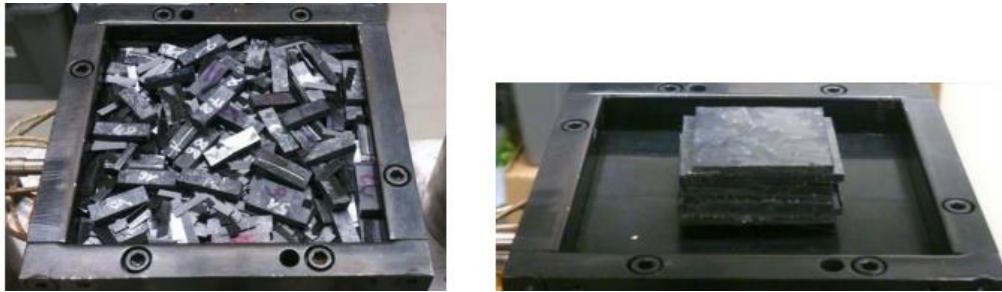
Figure 2-5. Mould cavity filled with 80 wt% SBS specimens and 20 wt% virgin strands (left). Stacked pieces of T-bracket flange at the mould cavity centre (right) [62].
