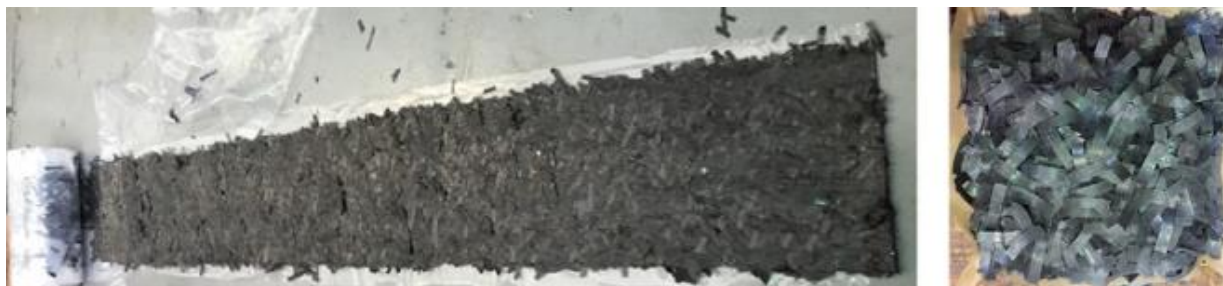
Figure 2-7. SMC sheet prepared from “fresh” prepreg trim waste tapes (left) and chopped “dry” prepreg trim waste tapes (right) [70].
