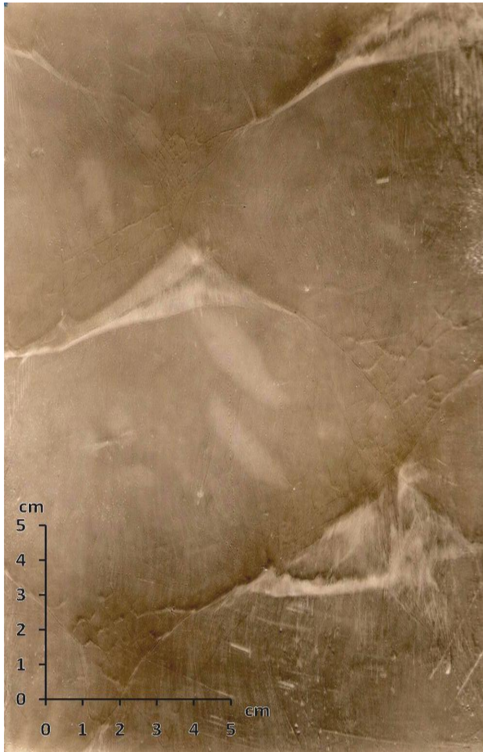
Figure 39: Smoked foil record of a detonation ( \text{CH}_4 + 2\text{O}_2 , p_0 = 7.5 kPa, 44 mm diameter round tube).
