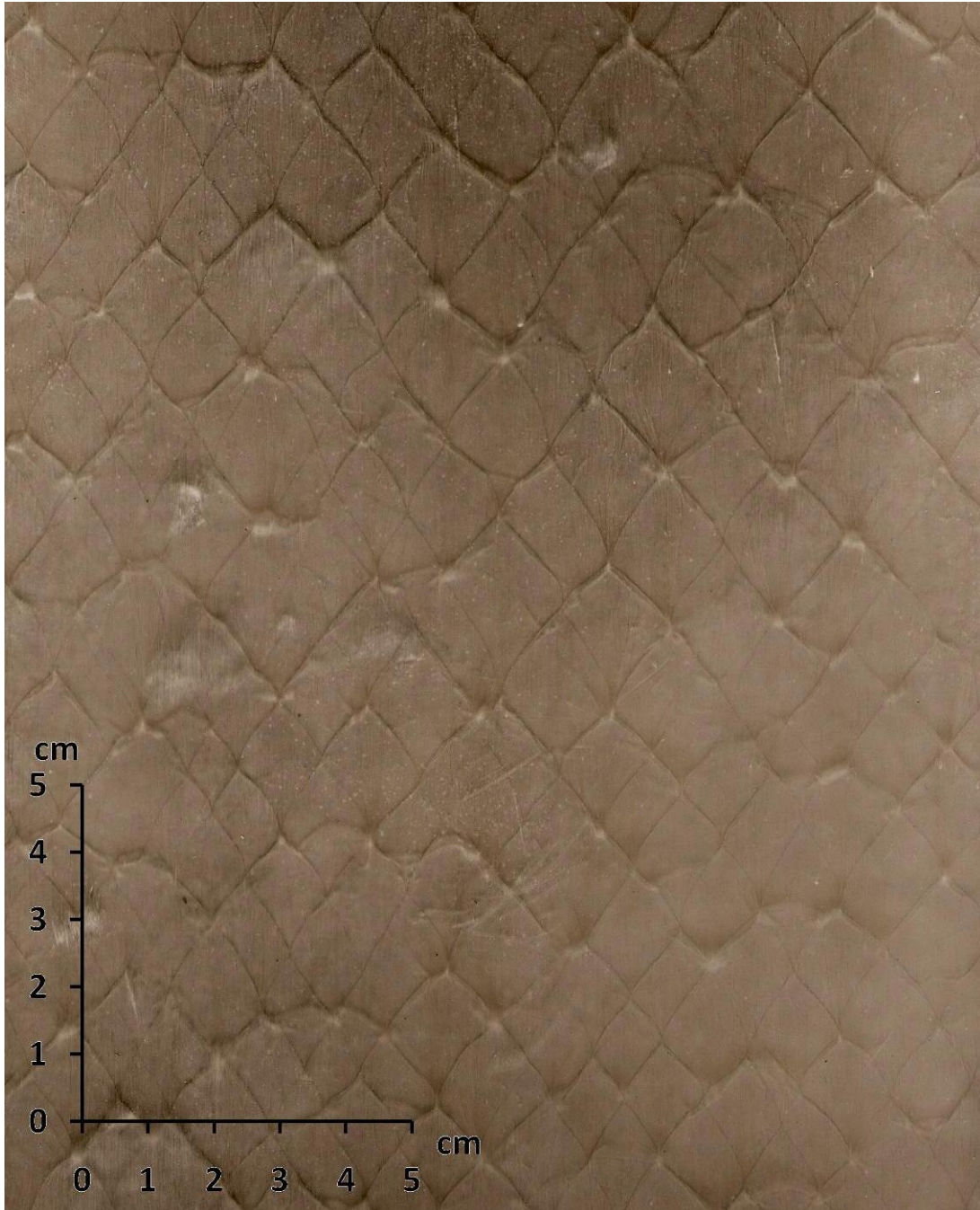
Figure 6: Typical smoked foil record of a detonation ( \text{C}_2\text{H}_2 + 2.5\text{O}_2 + 70\%\text{Ar} , p_0 = 10 \text{ kPa} , 58 mm diameter round tube).
