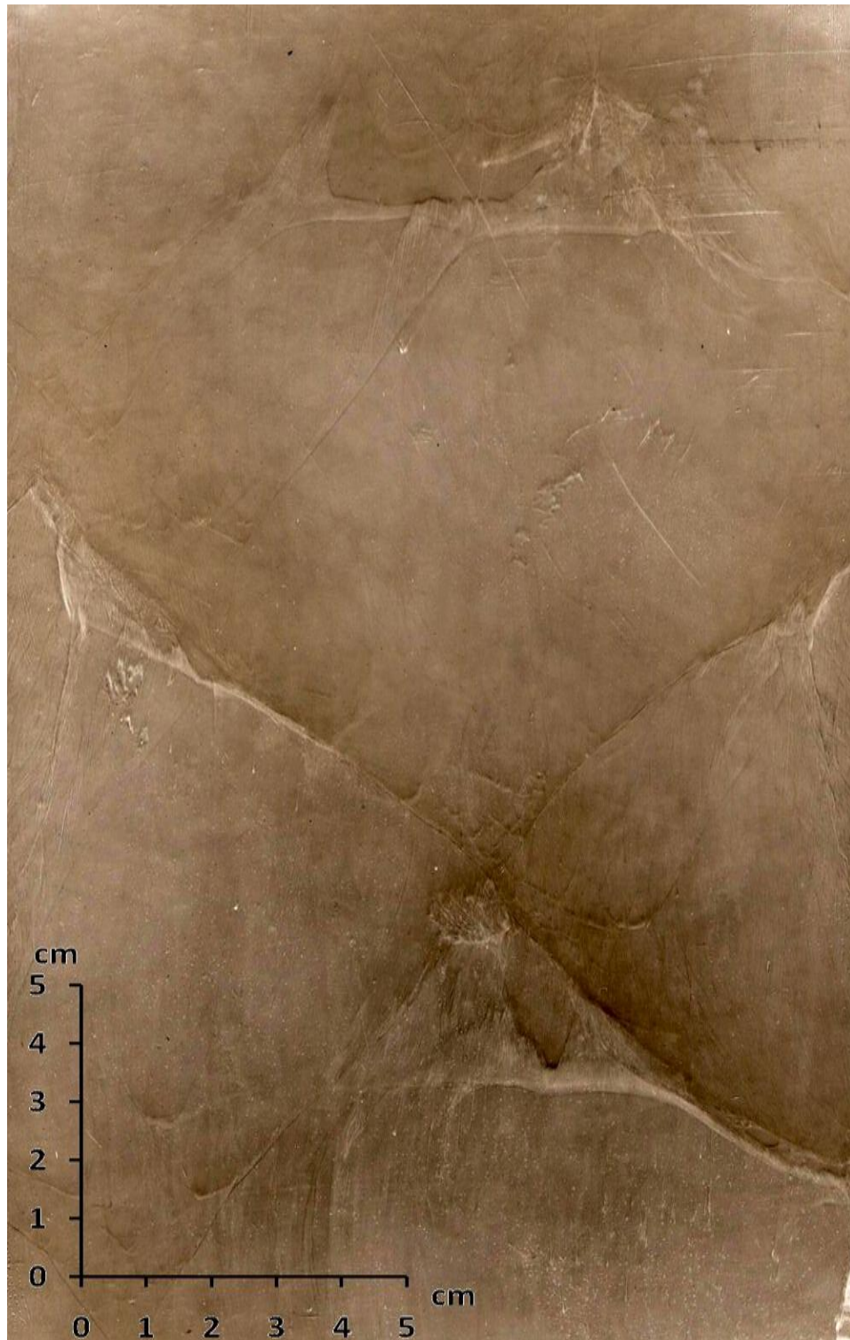
Figure 40: Smoked foil record of a detonation ( \text{CH}_4 + 2\text{O}_2 , p_0 = 4 \text{ kPa} , 44 mm diameter round tube).
