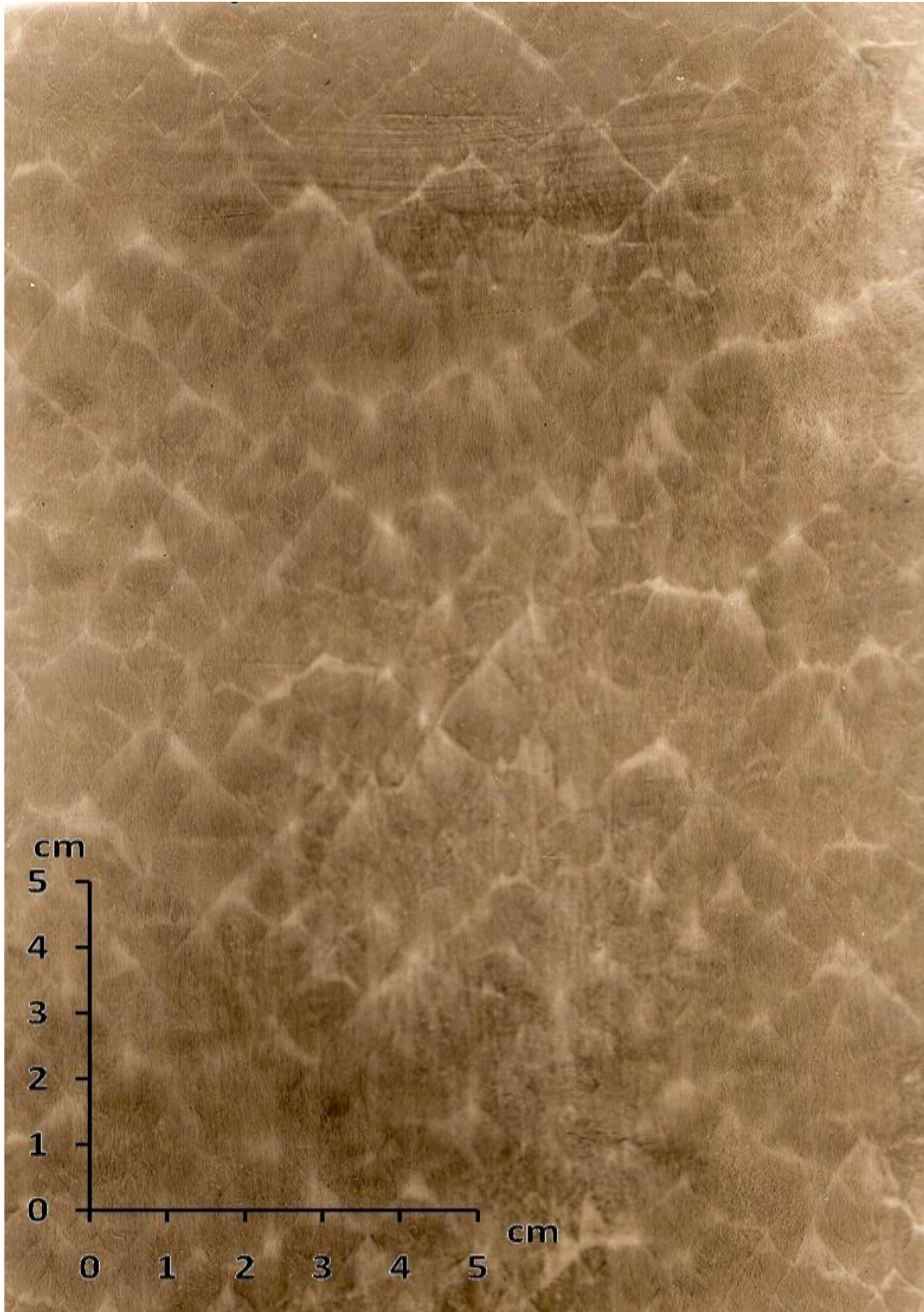
Figure 28: Smoked foil record of a detonation ( \text{CH}_4 + 2\text{O}_2 , p_0 = 35 \text{ kPa} , 44 mm diameter round tube).
