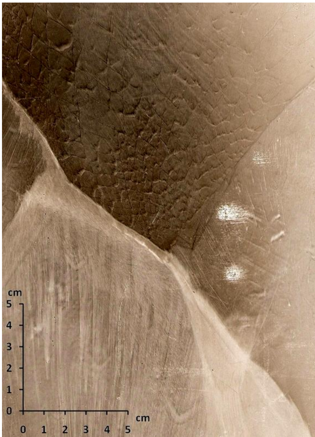
Figure 42: Smoked foil record of a detonation ( \text{CH}_4 + 2\text{O}_2 , p_0 = 8 \text{ kPa} , 3.175 mm channel).
