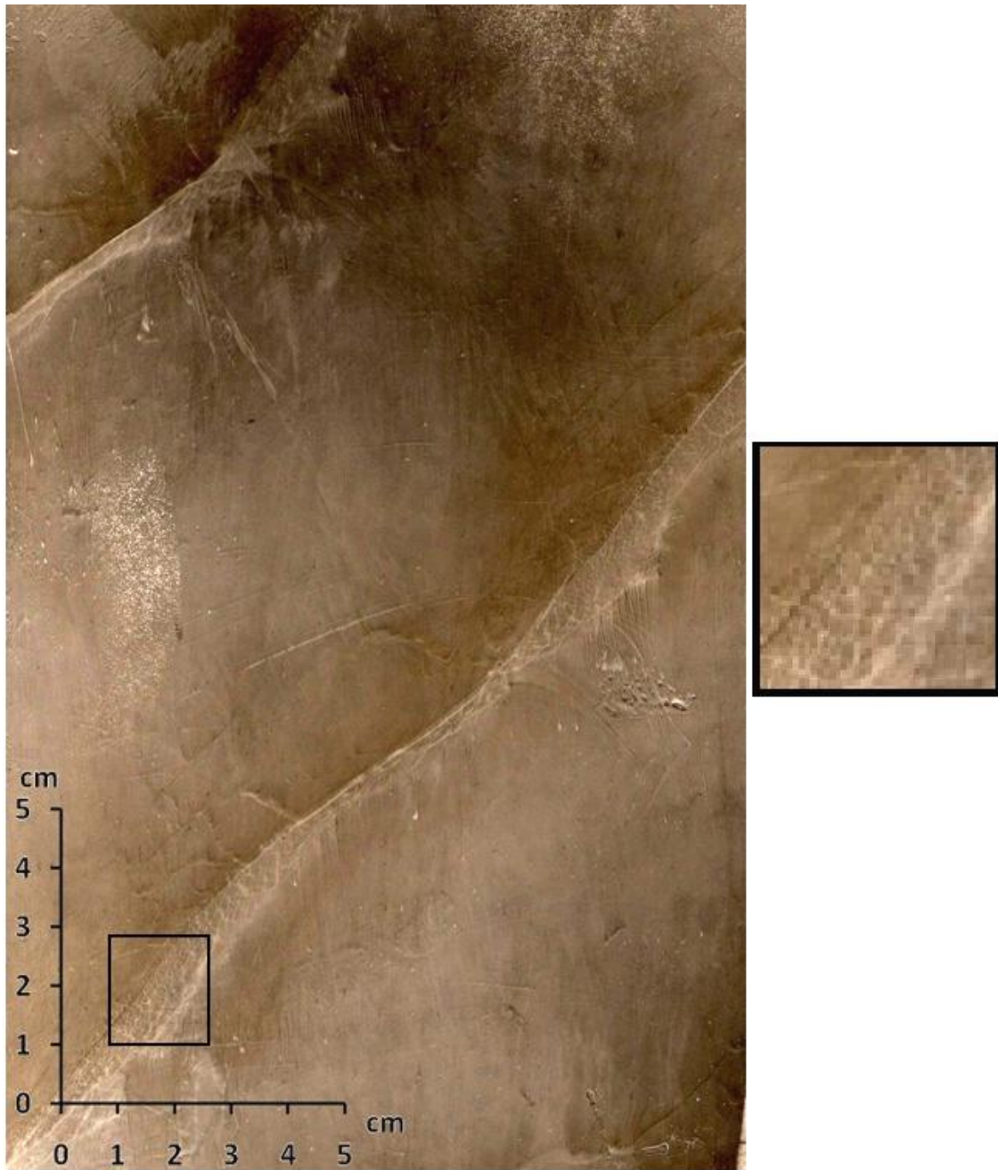
Figure 45: Smoked foil of a spinning detonation ( \text{CH}_4 + 2\text{O}_2 , p_0 = 3.25 kPa, 44 mm diameter round tube).
