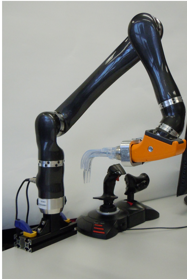
Figure 3–14: JACO arm, Pentax-AWS, and the joystick.
