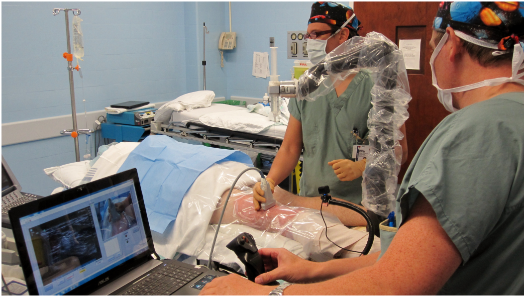
Figure 2-7: The Magellan robotic nerve block system.
