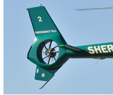
(b) EC 120B's shrouded tail rotor
