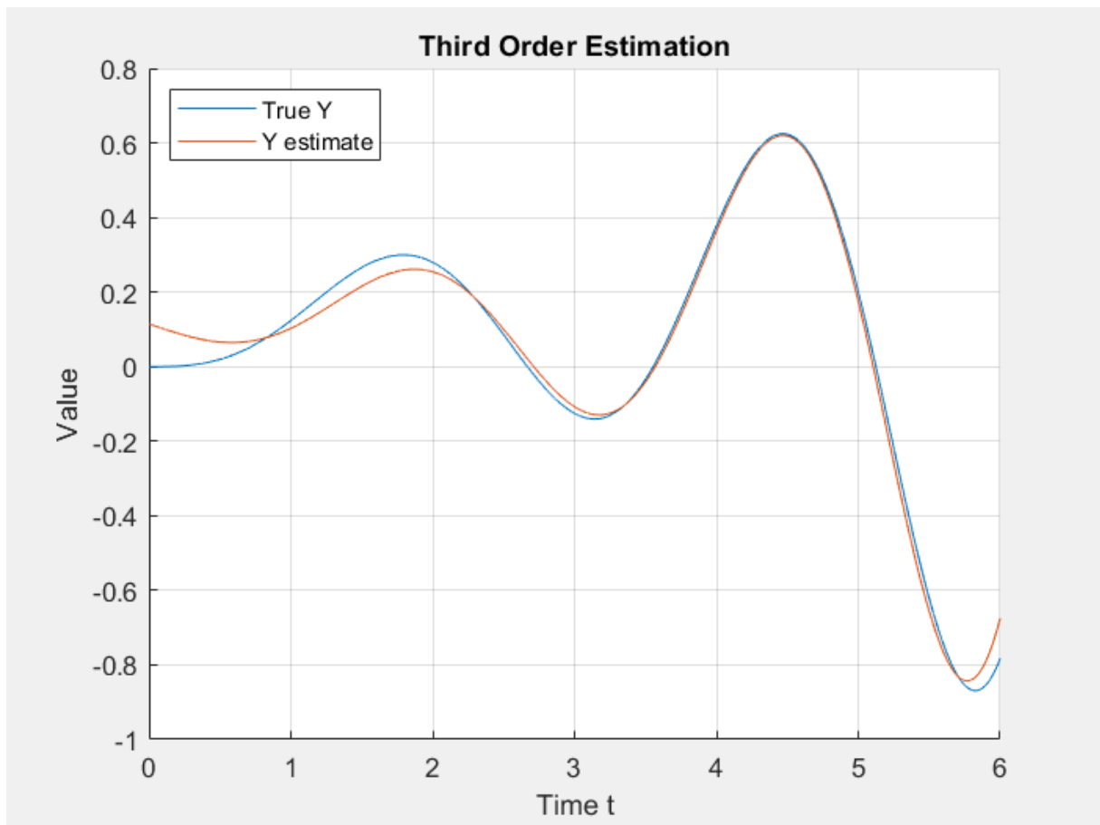
Figure 6: Estimate of y using third order vs. nominal y for noise of 1 SD (SNR -8.9652 dB)
