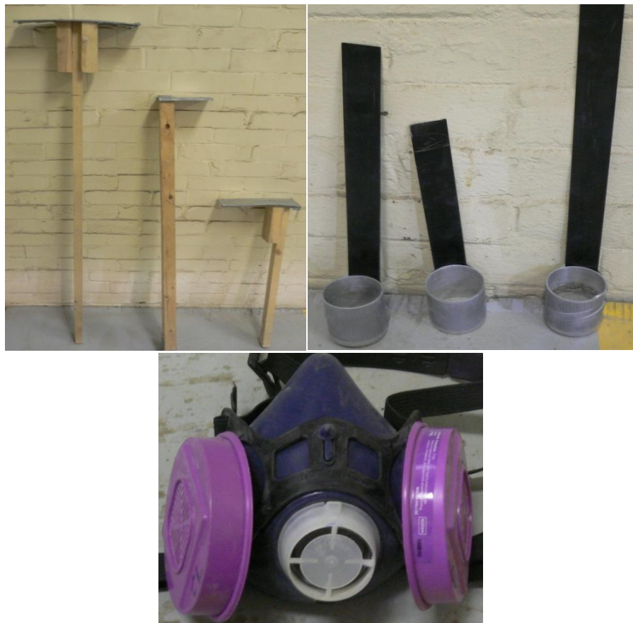
Figure 3.18: Testing equipment (clockwise from top left: tampers, sand samplers, dust mask)
