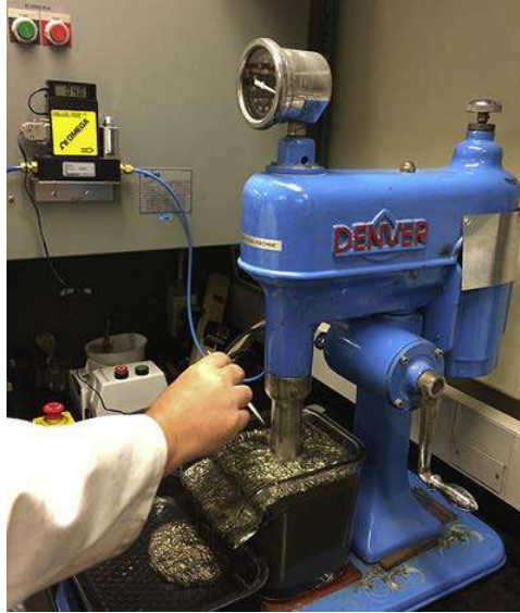
Figure 2.13 Batch flotation tests using a Denver Cell [15]
