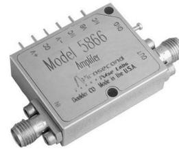
The Picosecond Pulse Labs Model 5866 amplifier has been designed to minimize the variations in gain and phase and to operate at very low frequencies. The 5866 includes internal temperature compensation for excellent output stability over temperature, and exhibits both high output and low power dissipation. It also incorporates internal sequencing circuitry, making it insensitive to power supply application sequence.
