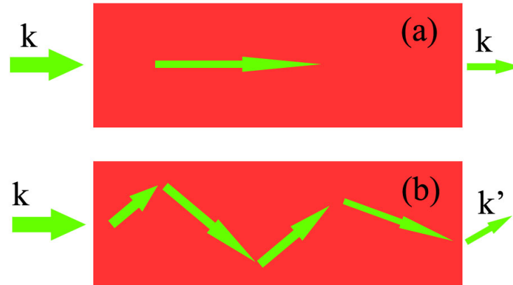
Figure 5.5: Schematic plot for illustrating specular transport (a) and diffusive transport due to random disorder scattering (b).
