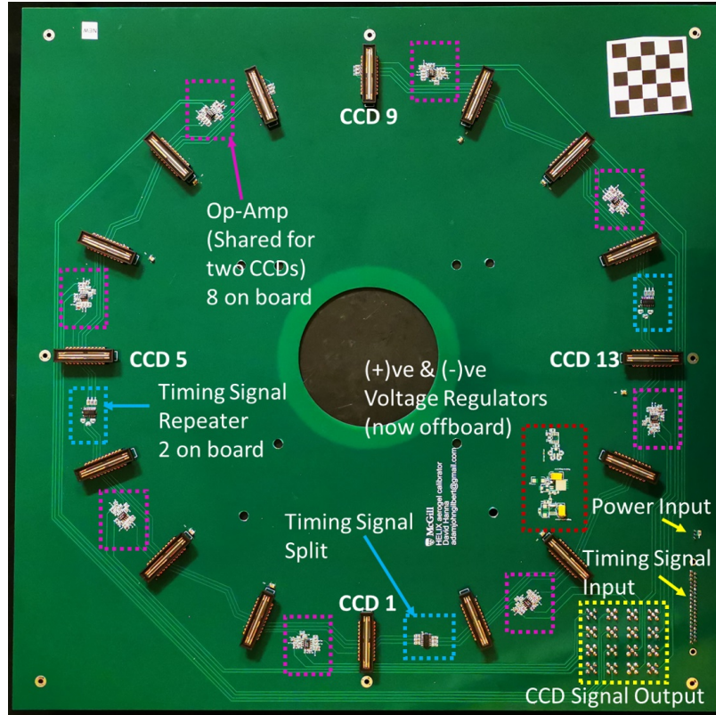
Figure 3–6: Diagram of the detection board designed and built by Adam Gilbert, an electrical engineer at McGill University, for this system. Any changes to the original board are given in the diagram in red, timing signal repeaters and splits are outlined in blue, the op-amps are outlined in magenta and the board connections for power, timing signal input and signal output are outlined in yellow.
