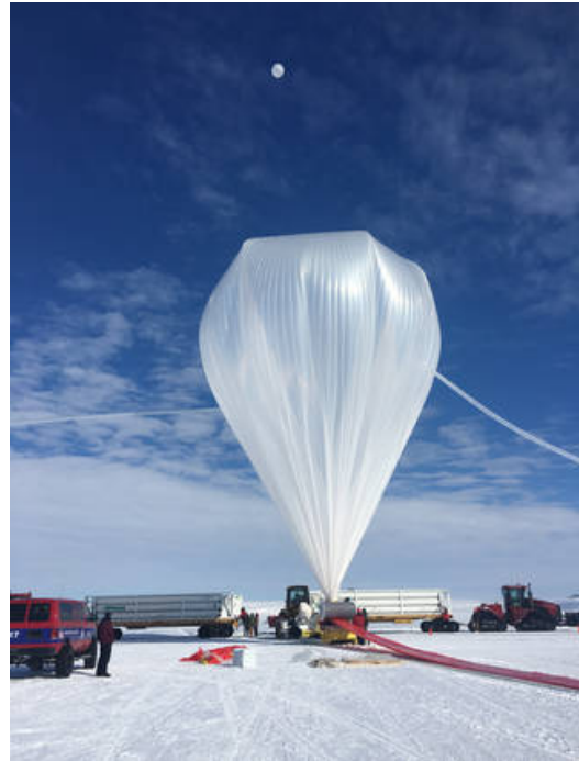
Figure 2–1: Partially filled balloon prepared to carry the STO-II payload during the 2016 balloon campaign. Image Source: [32].
