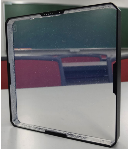
Figure 2-7: A picture of a flight quality aerogel tiles in its frame. Image Source: [39].
