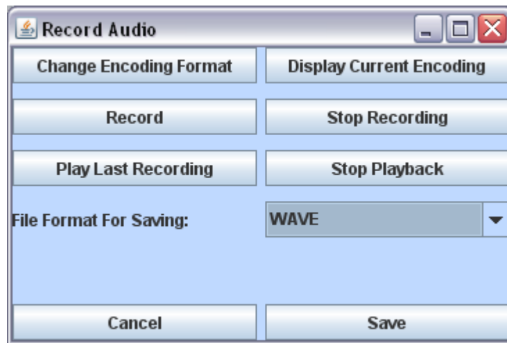
Figure 3.15: jAudio window allowing the user to record sound from a microphone or from the system sound in order to facilitate the testing of new features.
