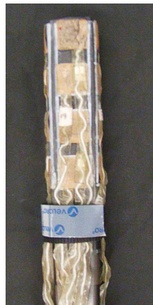
Figure 17 : Sensor configuration for upper hand on stick (adapted from Zane, 2012)
