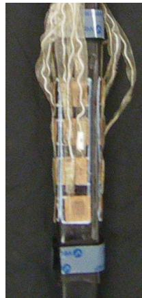
Figure 16 : Sensor configuration for lower hand on stick (adapted from Zane, 2012)
