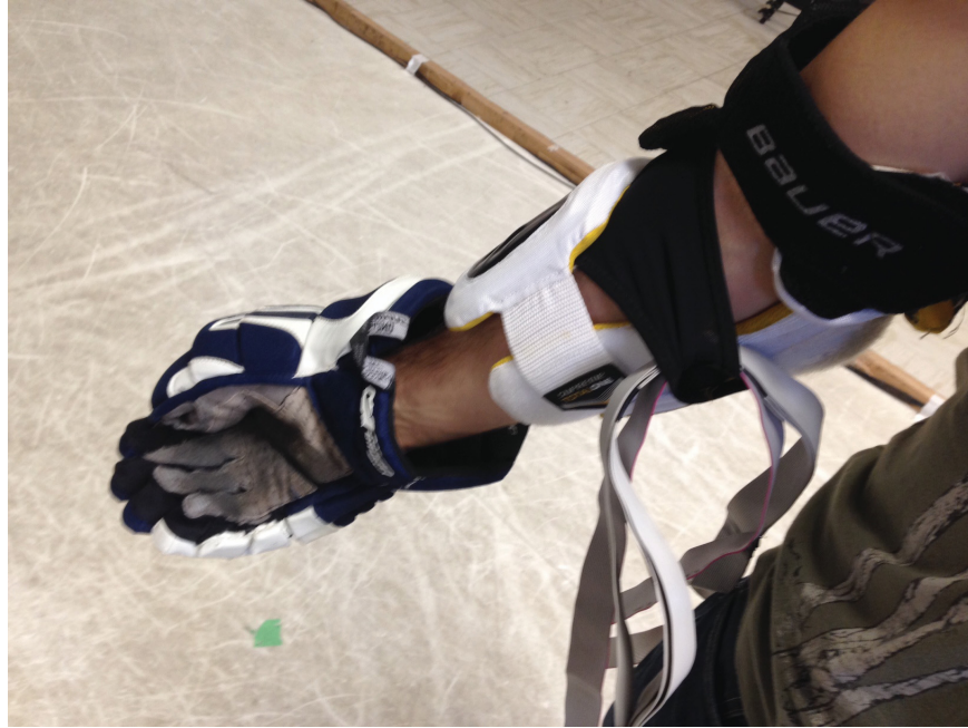
Figure 14 : Ribbon cable from strain gauges and FSA tethered to elbow pad to reduce interference during shooting tasks.
