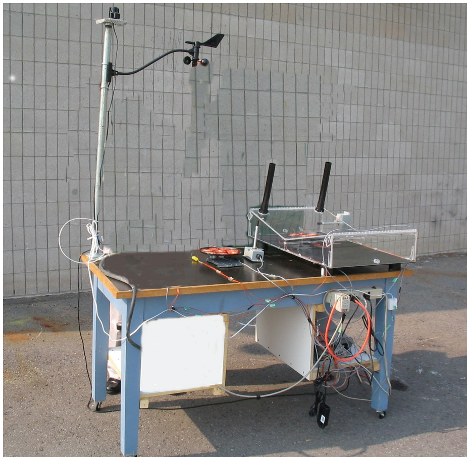
Figure 3.5. View of solar cabinet and open sun drying setup.
