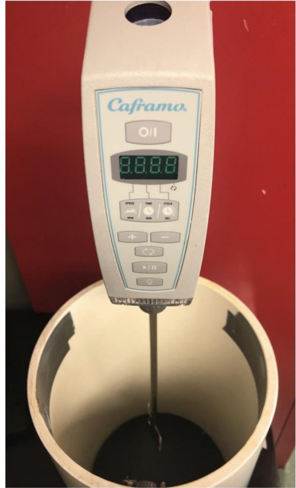
Figure S3.9. Pilot scale setup that can hold up to 20 L of synthetic wastewater. To measure TSS, microfiber, and microsphere removal, 100 mL samples were collected from the top valve approximately 3 cm from the surface of the water.
