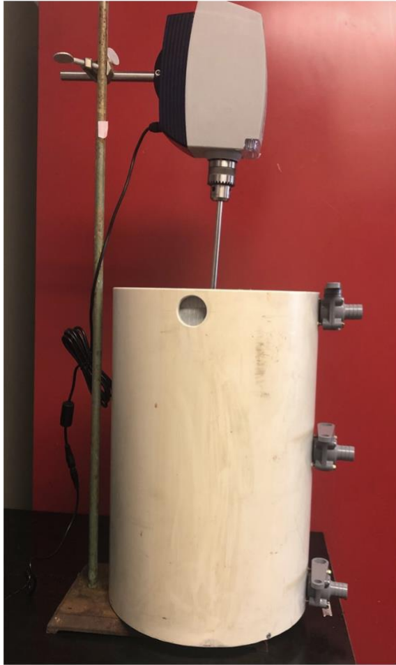
Figure S3.9. Pilot scale setup that can hold up to 20 L of synthetic wastewater. To measure TSS, microfiber, and microsphere removal, 100 mL samples were collected from the top valve approximately 3 cm from the surface of the water.
