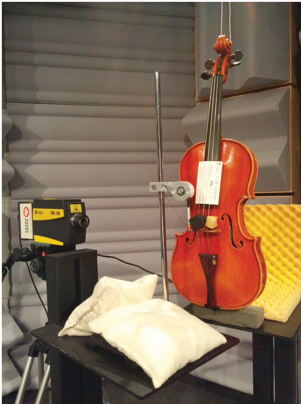
Figure 3.1: The experiment setup in the Spatial Audio Laboratory. From left to right are: the laser vibrometer, the hammer and pendulum secured on an altazimuth mount, and the violin suspended from the ceiling and gently supported by foam.
