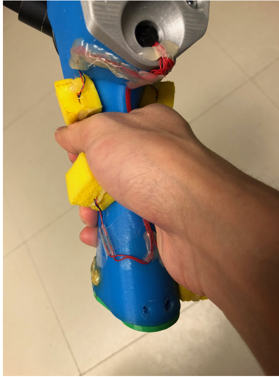
Fig. 3.3: Different contact points between the motor discs and a user's hand.
