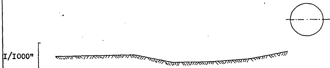
FIGURE 11. SURFACE TRAVERSE OF A LATHE PREPARED LIMESTONE SPECIMEN PROCEDURE NO.3. RE. TABLE E.9.I.
