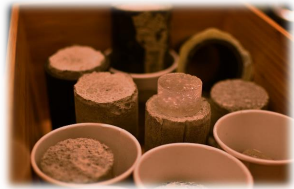
Figure 3: Cured Aircrete samples and transparent mortar samples
