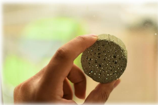
Figure 2: Light transmitting Aircrete disk cured in final batch
