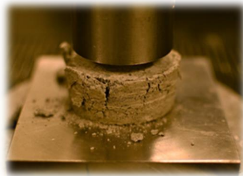
Figure 5: Crushed Aircrete sample under the Instron universal testing machine
