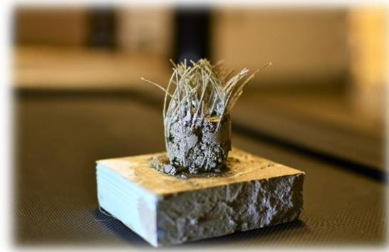
Figure 1: Cracked fiber embedded Aircrete from first trial
