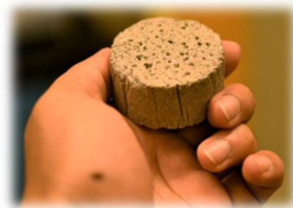
Figure 4: Light transmitting Aircrete disk cured in final batch
