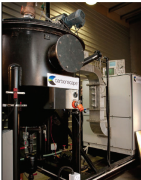
Figure 2.10: Carbonscape's demonstration microwave pyrolysis unit (Carbonscape, 2012)
