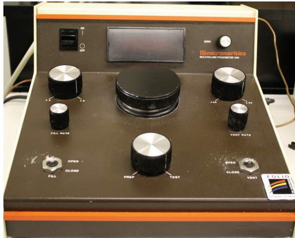
Figure 6.2: Helium Pycnometer (Model 1305 Multivolume, Micromeritics Instrument Corporation, Norcross, GA)
