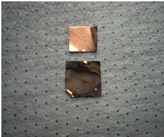
Figure 4.6: Picture of bare Cu foil (top) and graphene-covered Cu foil (bottom).
