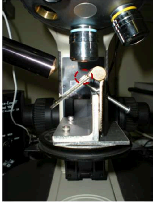
Figure 3.7: Experimental setup for angle detection measurements. The dashed circle is the substrate lying on the tilted stage and the stage's angle is adjusted with the screw.
