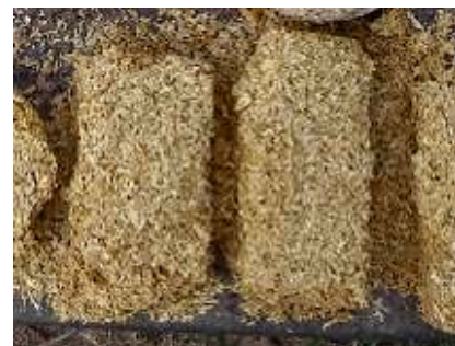
Figure 43: Collapsing of sides and corners
