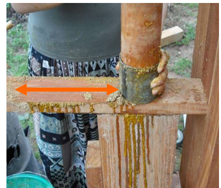
Figure 52 Wood plank on stand supporting dye in filling and briquetting positions
