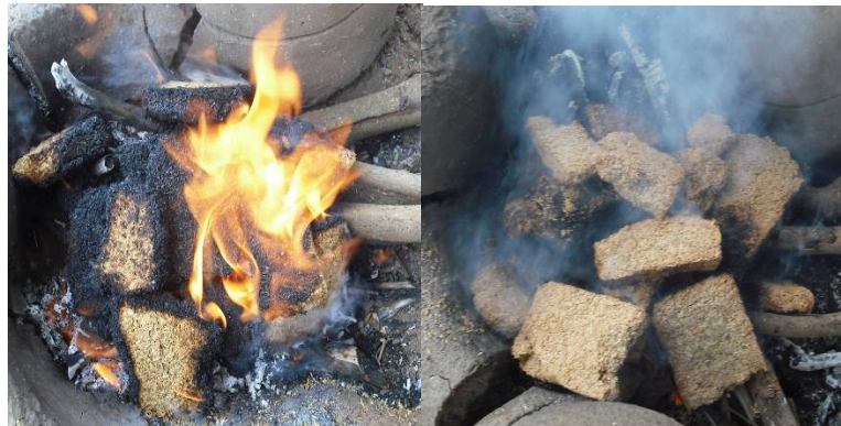
Figure 46a Combustion of an oil briquette
