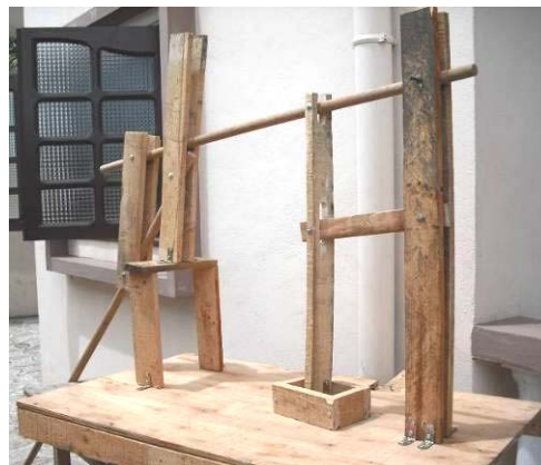
Figure 37b : Double-lever prototype
