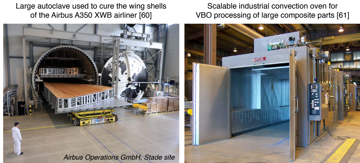
Fig. 1-4. Typical industrial equipment used to cure advanced composite aero-structures (from: [50, 51]).
