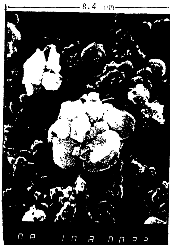
Fig. 52 SEM microphotographs of the non-mags. Lead particles are identified with a lead X-ray map (particles showing the white dots.), right side pictures.
