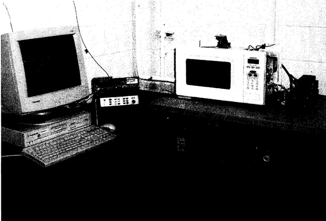
**Figure 3.2** Photograph of the microwave drying setup showing cavity, air heating and blowing system, display panels, triac power regulator, filament transformer, strain gauge, and data acquisition system
