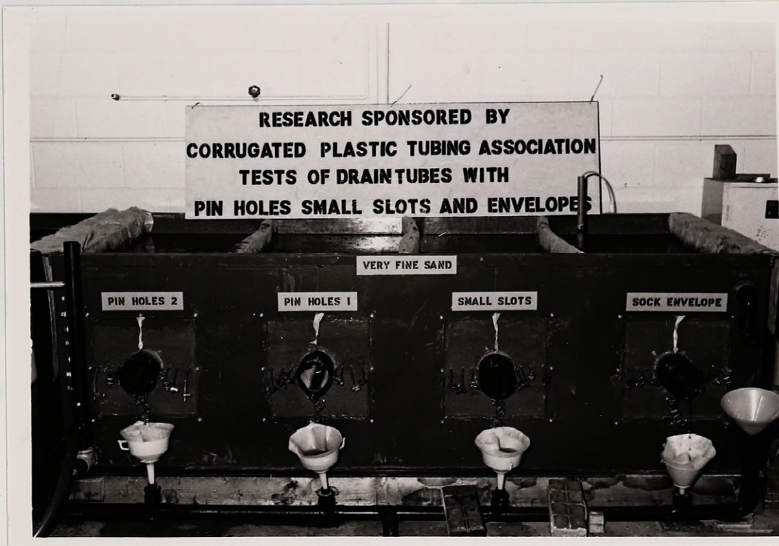
Photograph 1. Test tank no.3 with 4 drain tubes functioning in fine sand. Note, the overflow water level controls at each end of the tank.
