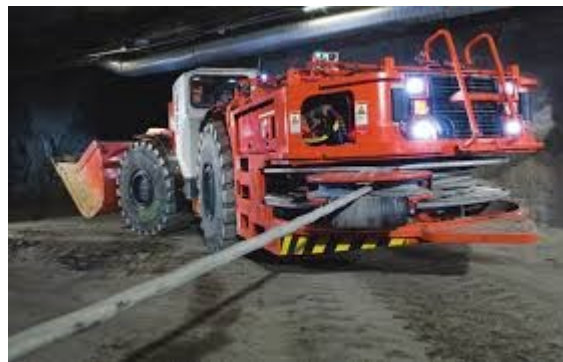
Figure 3) Tethered Electric LHD (Mining Magazine 2017)
