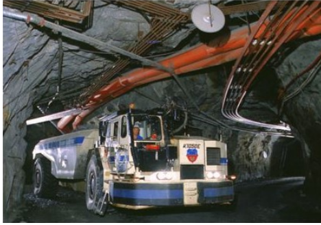
Figure 2) Trolley Electric Truck (Queen's University, Electric equipment 2017)
