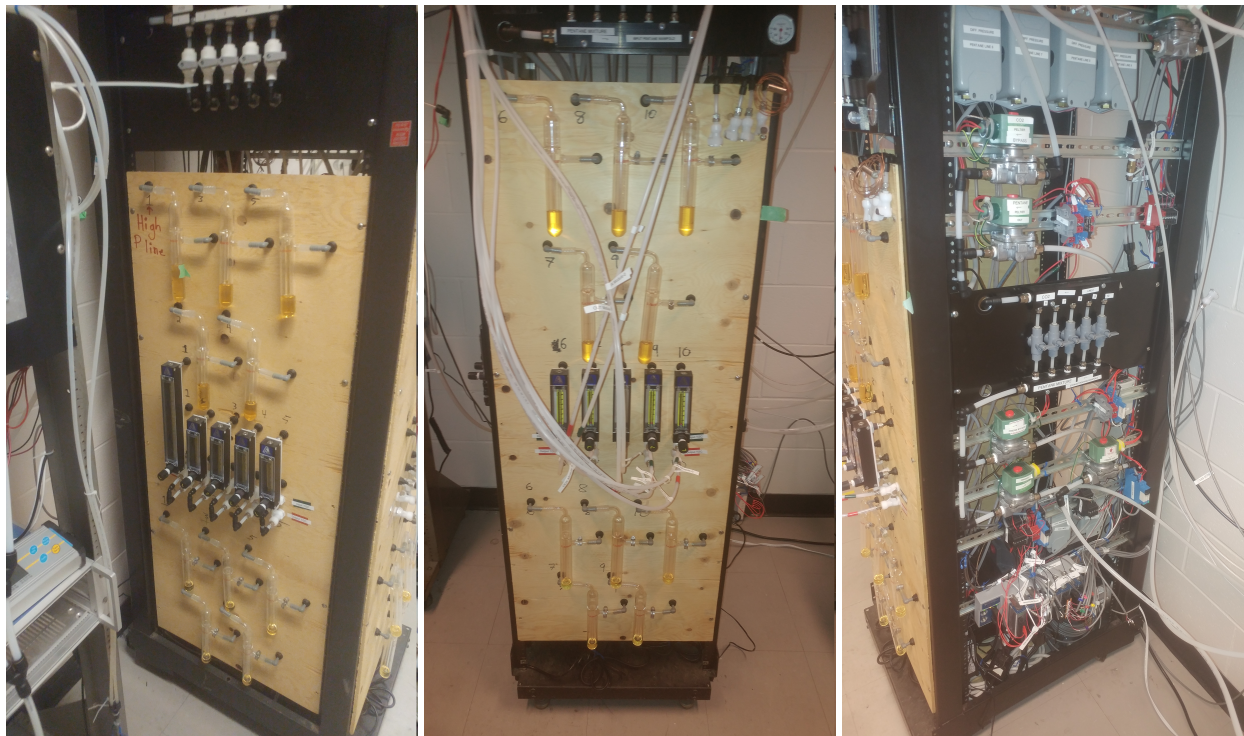
Figure 4.4: The three sides of the custom gas system designed for the McGill sTGC testing lab. The gas system mixes \text{CO}_2 and pentane into the proportions needed for proper operation of the sTGC quads. Left and Middle shows the bubblers, rotameters and manifold valves of the 10 independent lines. Right shows the solenoid valves and electronics for the data acquisition system [57].
