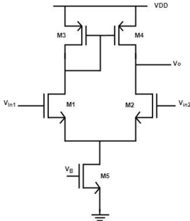
**Figure 2.11** – Differential amplifier with current mirror load
