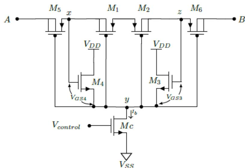
**Figure 2.23** – Linear Current Controlled Pseudo-Resistor printed with permission from [57]
