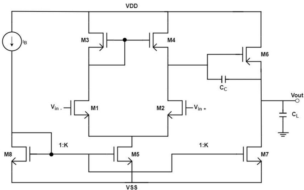
Figure 2.15 – Two – Stage OTA schematic
