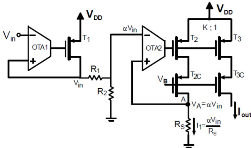
**Figure 2.4** – Voltage attenuation VI converter implementation reprinted with permission from [2] (Copyright © 2011, IEEE)
