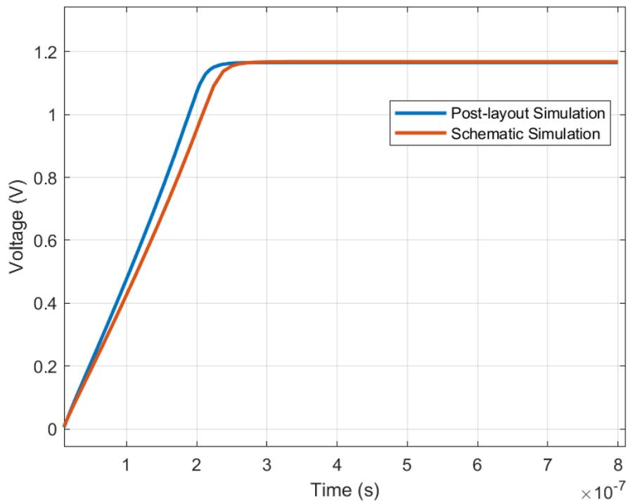
**Figure 3.13** – Step response comparison of schematic and post-layout simulation
