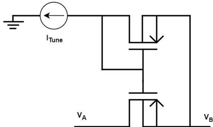
**Figure 2.22** – Current Controlled Pseudo-Resistor
