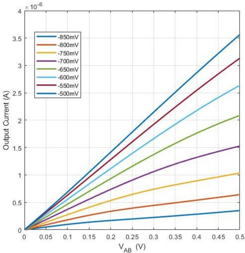
**Figure 4.7** – Voltage  $V_{AB}$  with varied current biases for different resistances
