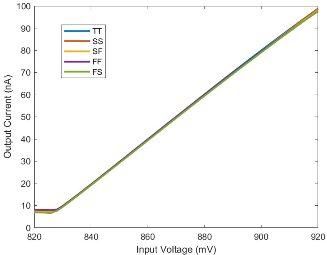
**Figure 5.16** – Output current over the different process corners
