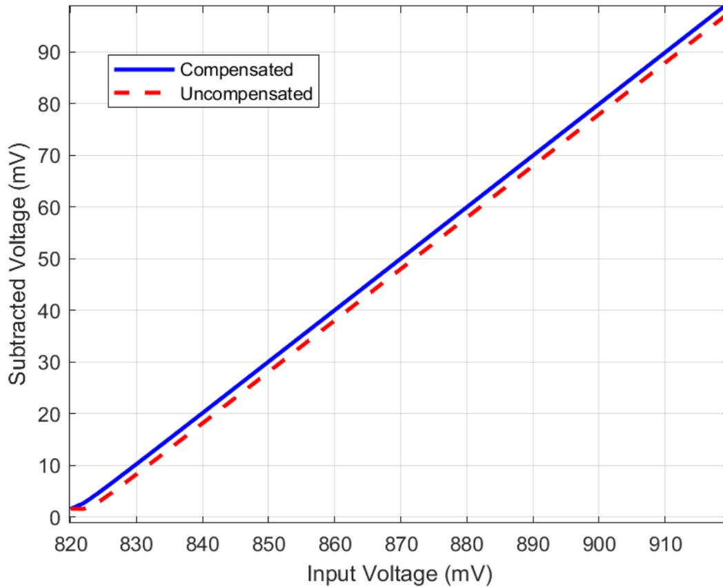
**Figure 5.3** – Output of the voltage subtractor with and without compensated subtracted values
