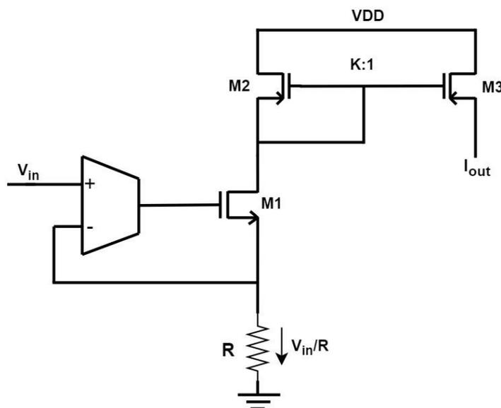
**Figure 2.3** – Voltage to current converter using an OTA in negative feedback with an output current mirror where the conversion occurs at  $R_S$
