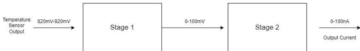
**Figure 1.1** – High level VI converter overview
