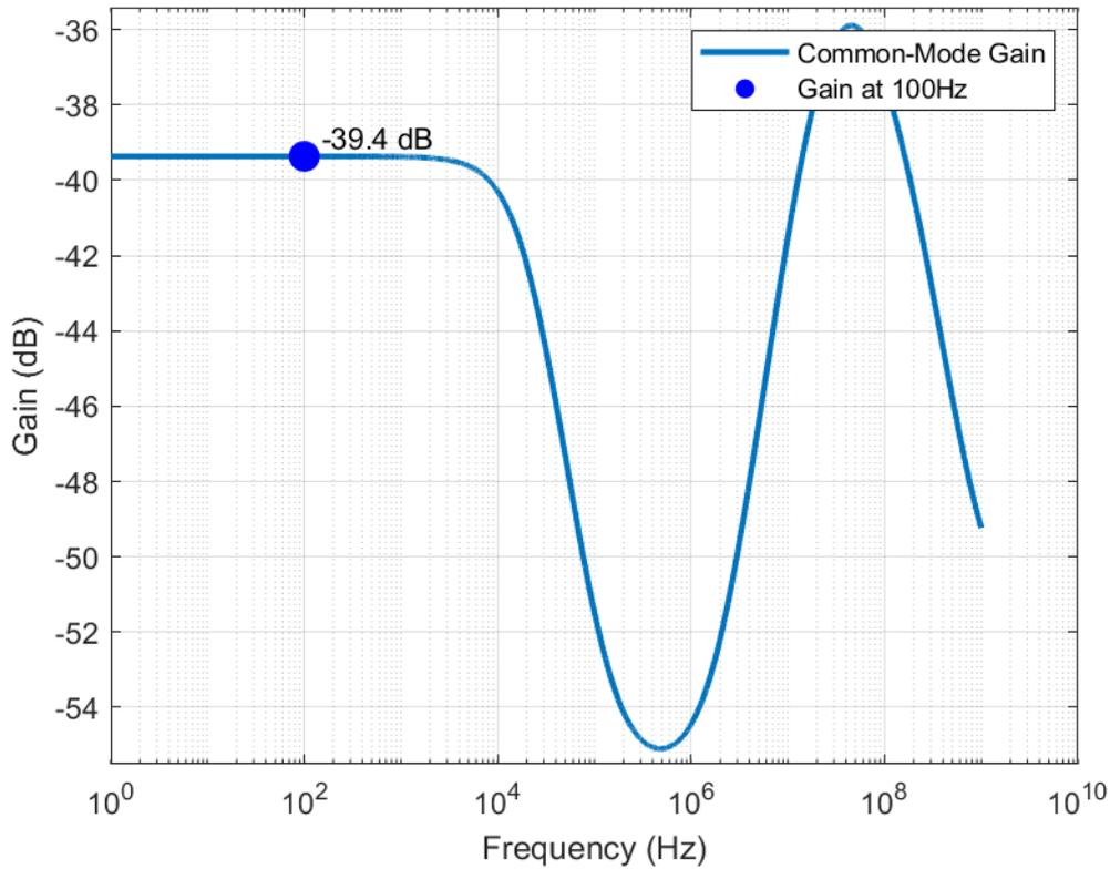
**Figure 3.8** – Common-mode gain plot
