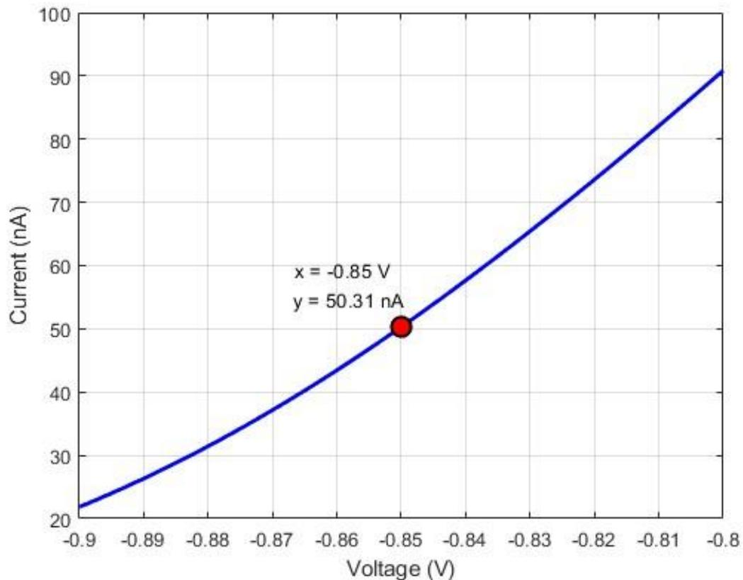
**Figure 4.4** – Output current when bias voltage for current source is varied with a  $50\text{mV}$  input to terminal A
