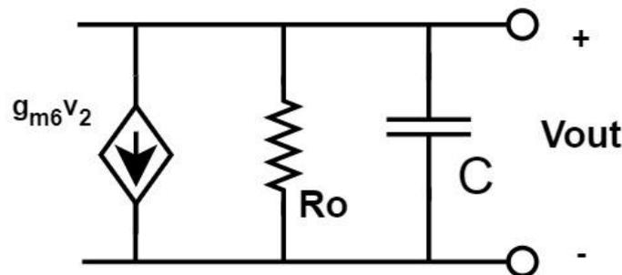
**Figure 2.16** – Simplified small signal model of the second stage
