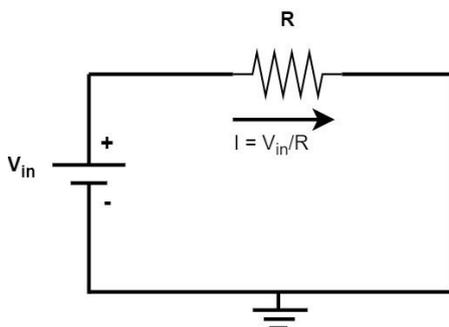
**Figure 2.2** - Basic VI converter using only a resistor with the current flowing through the circuit being proportional
