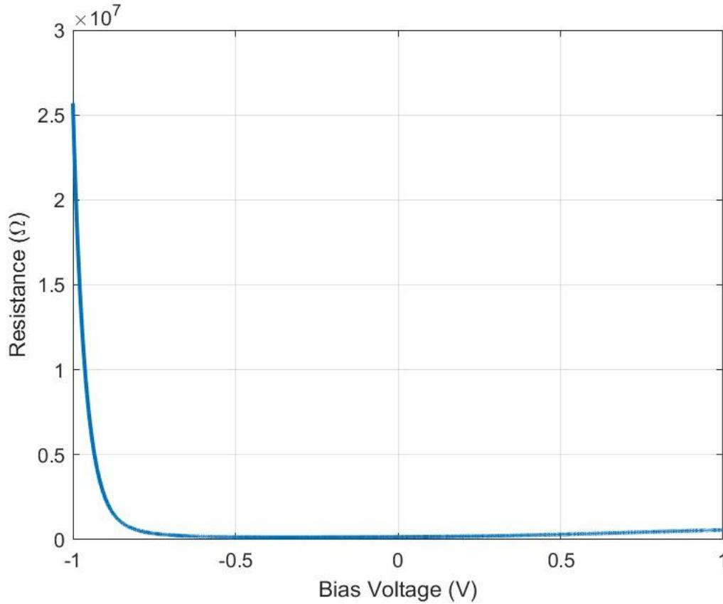
**Figure 4.8** – Resistance seen from pseudo-resistor with varying bias voltage
