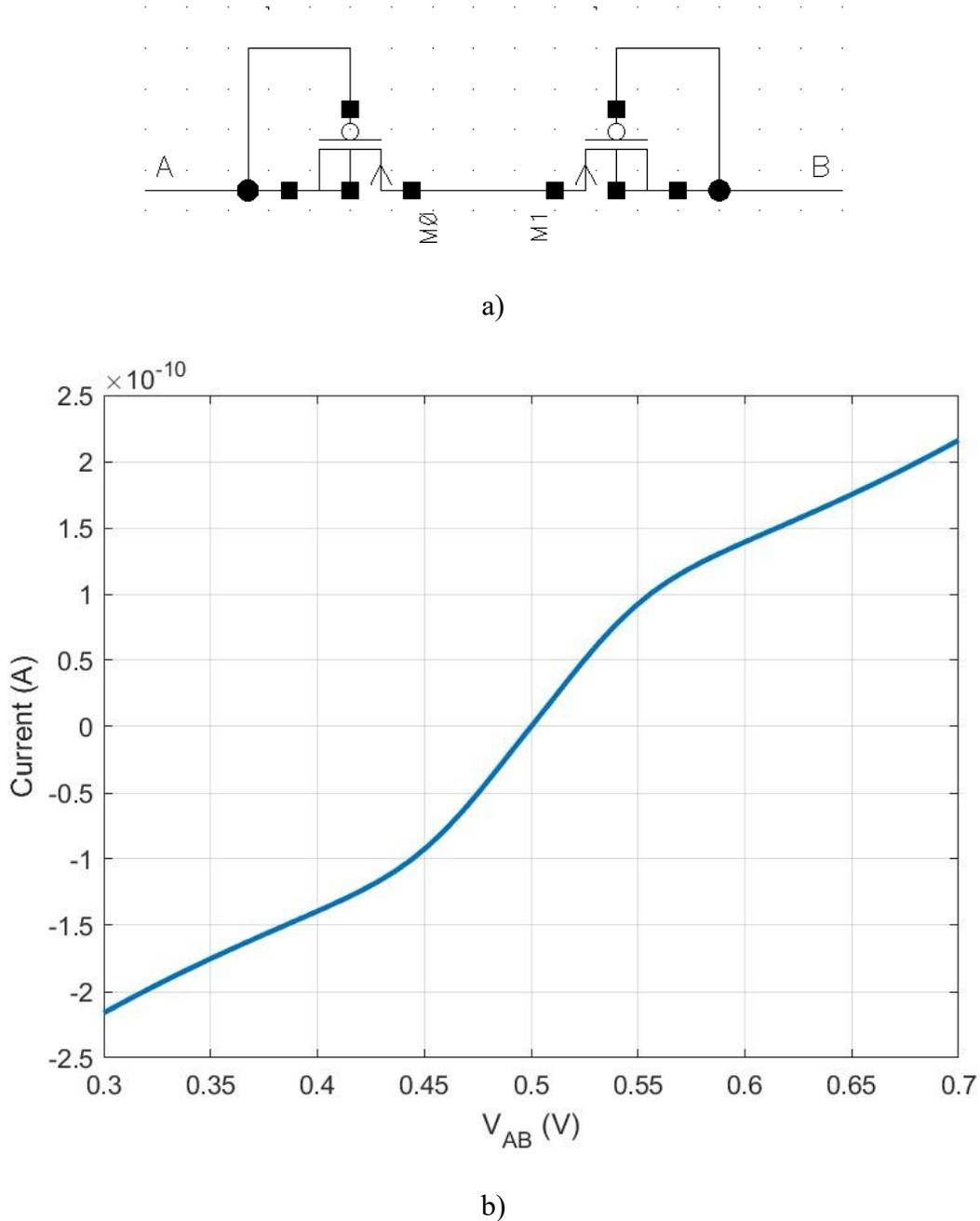
**Figure 4.3** – a) multi-cell pseudo-resistor with symmetry and variable  $V_{GS}$ , b) I-V characteristics of a)
