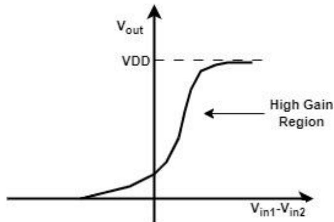
**Figure 2.12** – Large signal input and output characteristics
