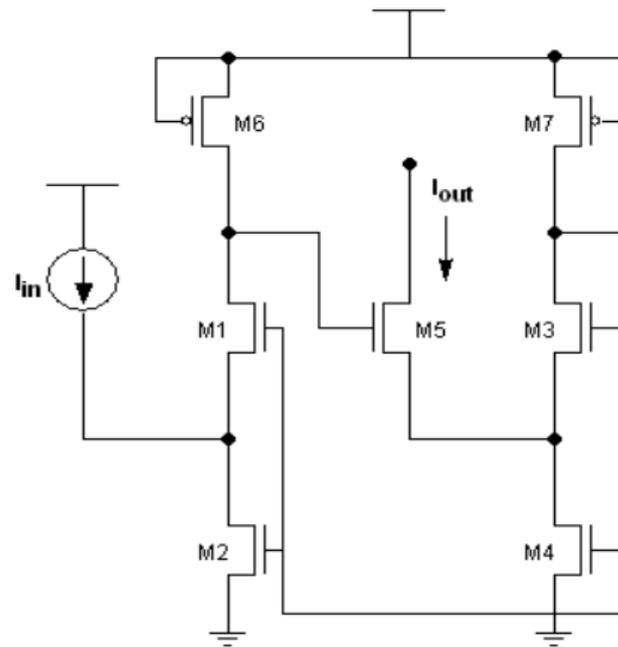
**Figure 2.8** – Current mirror topology reprinted with permission from [15] (*Copyright* © 2011, IEEE)
