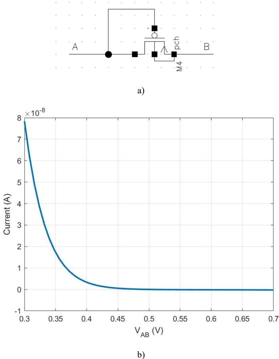
**Figure 4.1** – a) Test circuit for a single cell PMOS pseudo-resistor, b) I-V characteristics with respect to a varying drain voltage
