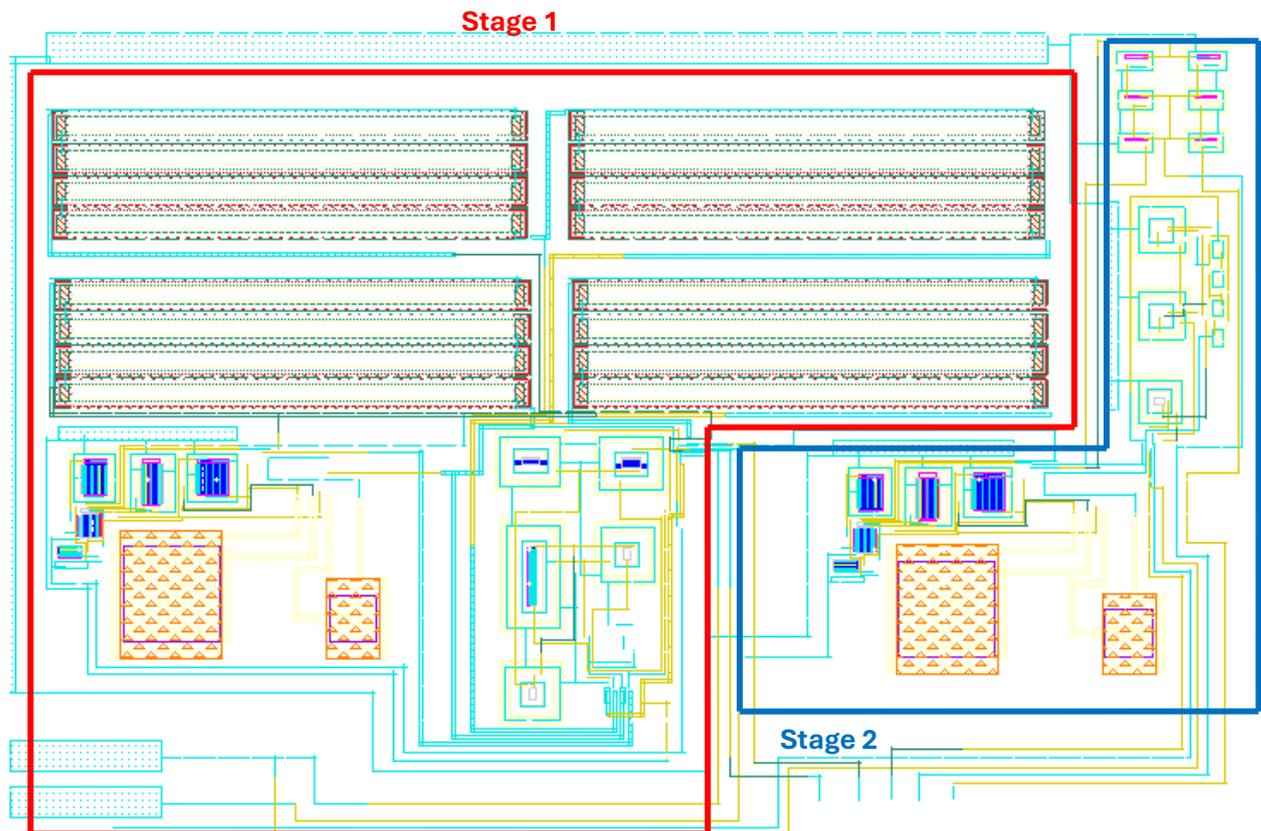
**Figure 5.12** – Full VI Converter layout
