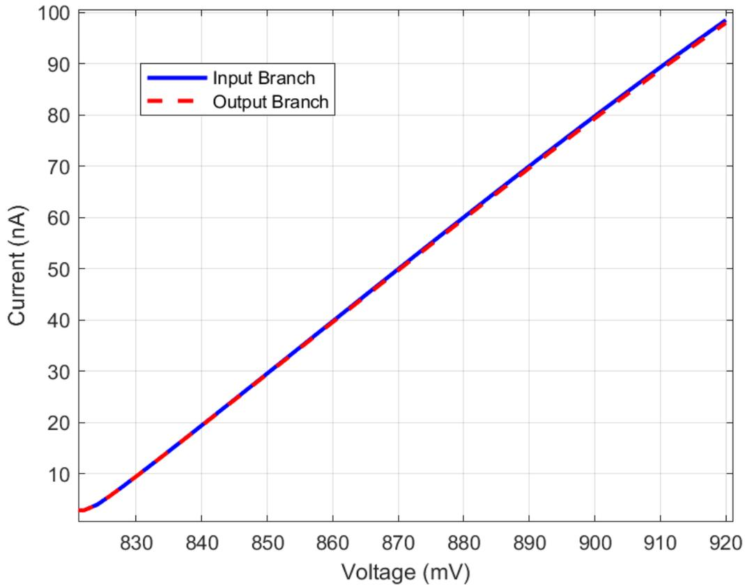
**Figure 5.11** – Comparison between input and output branch of the current mirror
