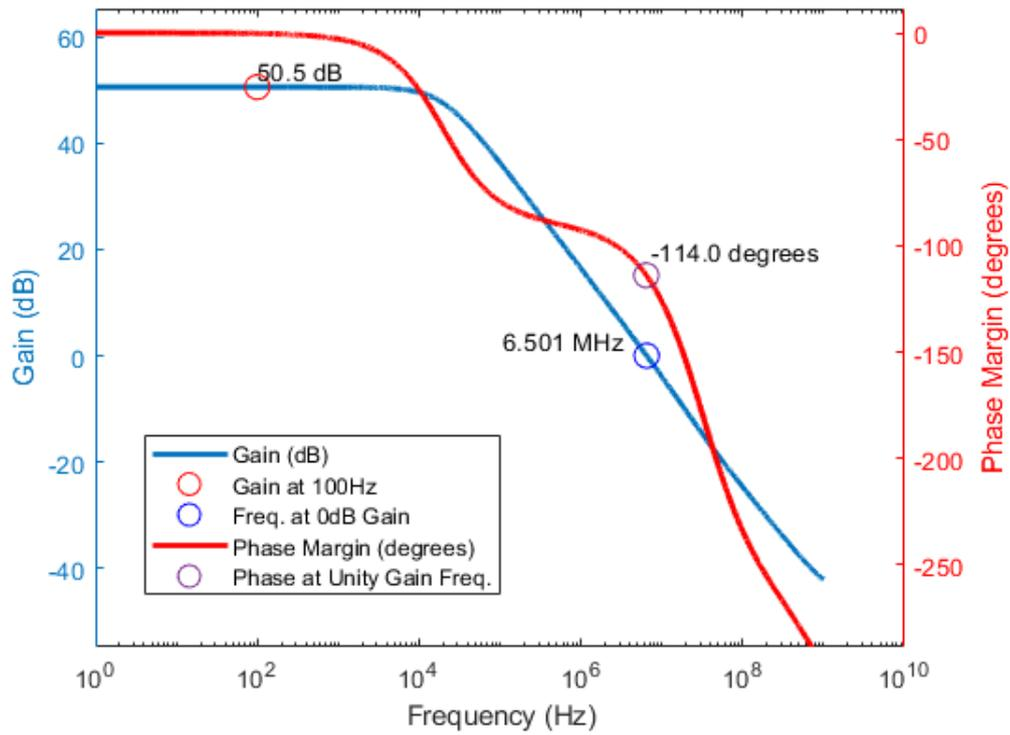
**Figure 3.12** – Post-layout gain and phase plot
