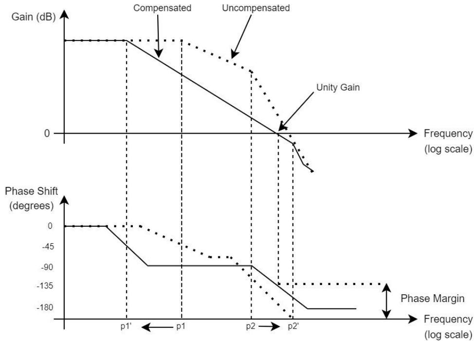
**Figure 3.5** – Gain and phase plots with pole splitting
