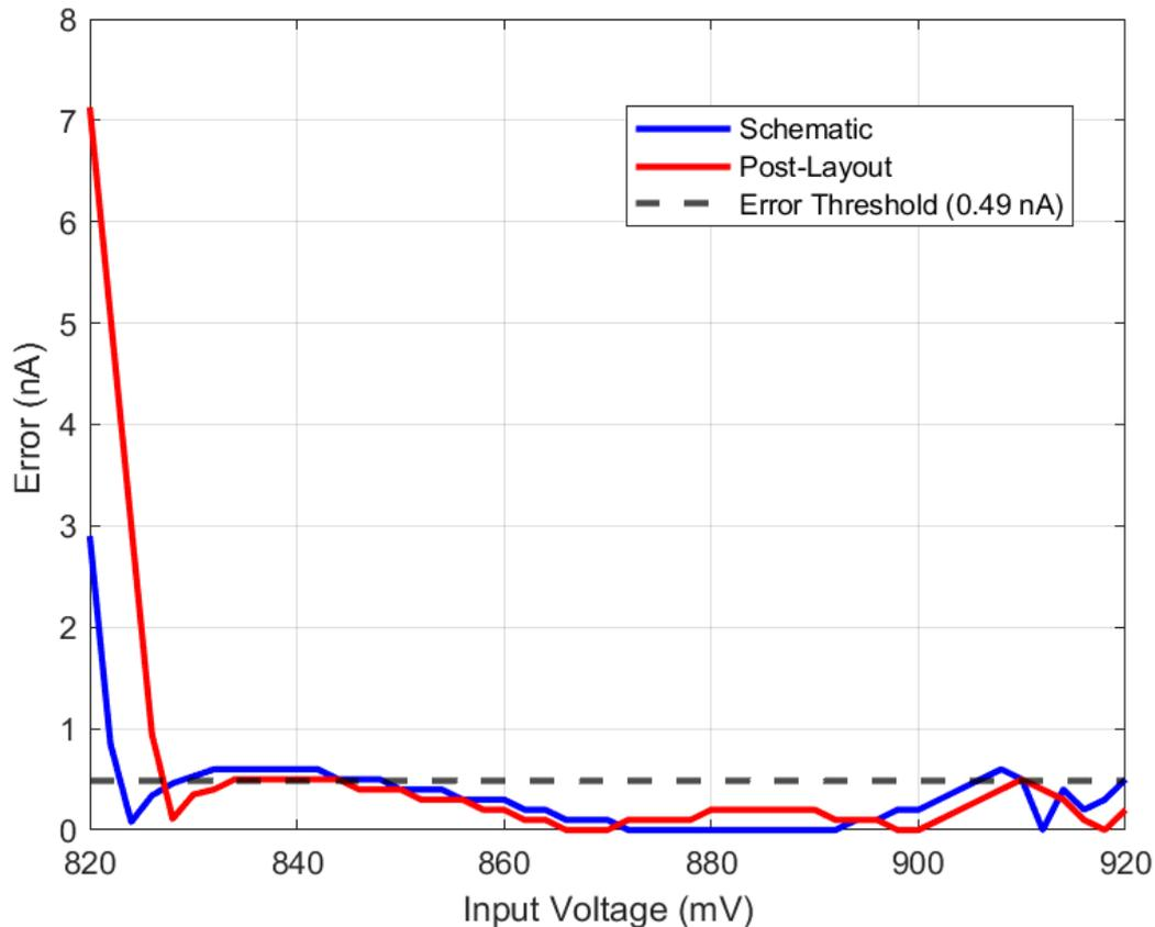
**Figure 5.14** – Absolute error in  $nA$  vs input voltage for schematic and post-layout simulation
