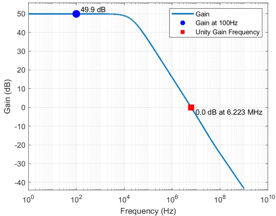
**Figure 3.6** – Open-loop gain plot
