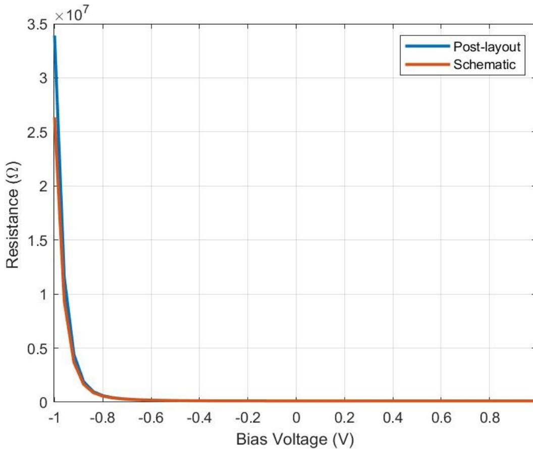
**Figure 4.15** – Resistance Range for schematic and post-layout
