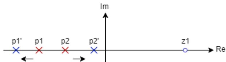
**Figure 3.4** – Pole Splitting in the complex frequency plane
