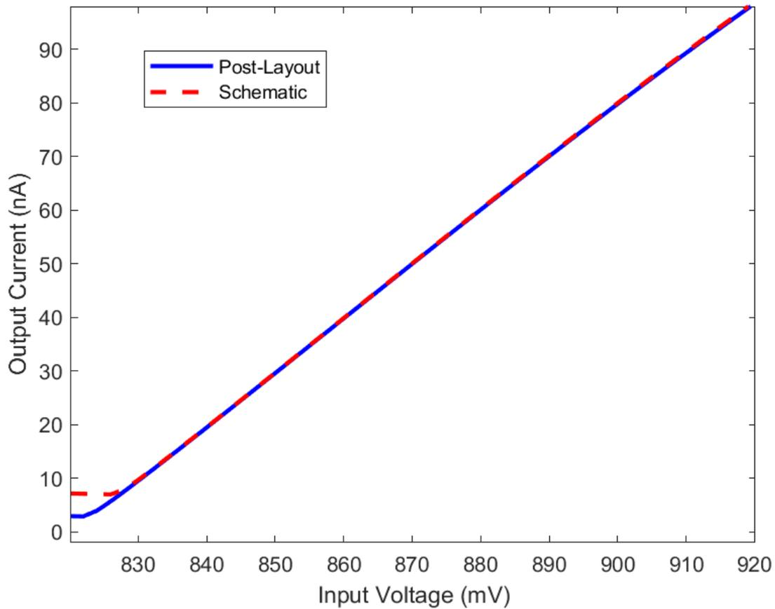
**Figure 5.13** – Schematic vs post-layout comparison of output current with 500mV load voltage
