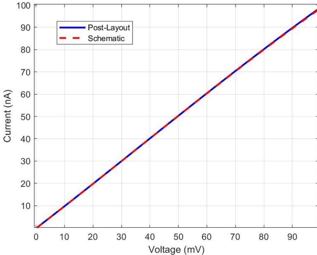
**Figure 4.13-** Output current vs Input voltage comparison for schematic and post-layout
