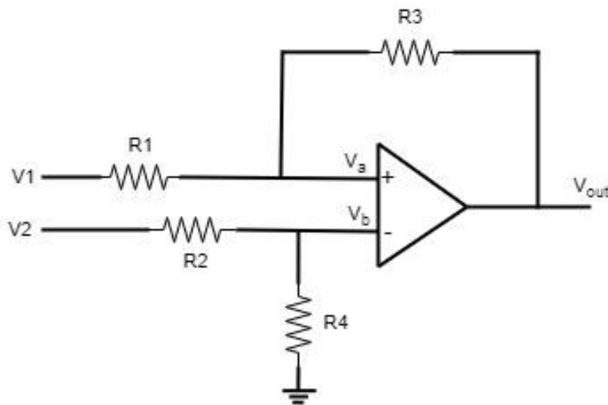
**Figure 5.2** – Difference amplifier circuit
