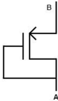
**Figure 2.19** – PMOS in diode configuration
