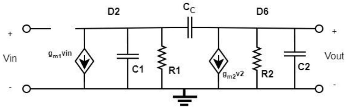
**Figure 3.3** – Small signal model with compensation
