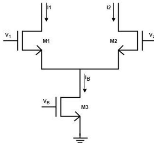
**Figure 2.9** – Differential pair circuit
