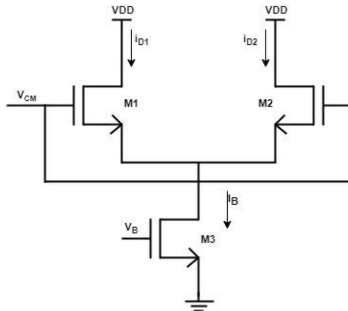
**Figure 2.10** - Differential amplifier in a common-mode configuration
