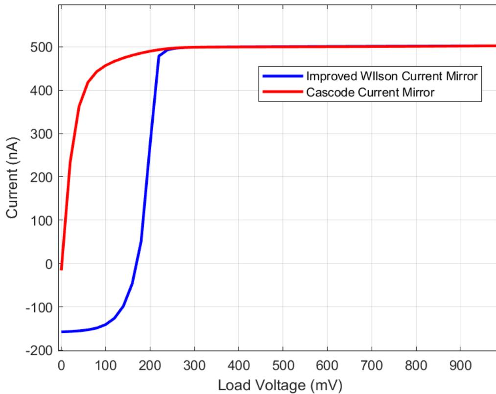
**Figure 5.7** – Comparing the Improved Wilson current mirror vs cascode current mirror with a varied output load voltage
