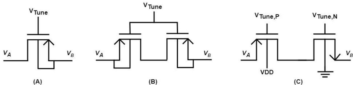
**Figure 2.21** – Voltage controlled pseudo-resistor structures: (a) voltage controlled single MOS pseudo-resistor; (b) voltage-controlled series connected MOS pseudo-resistor structure; (c) CMOS voltage controlled pseudo-resistor structure
