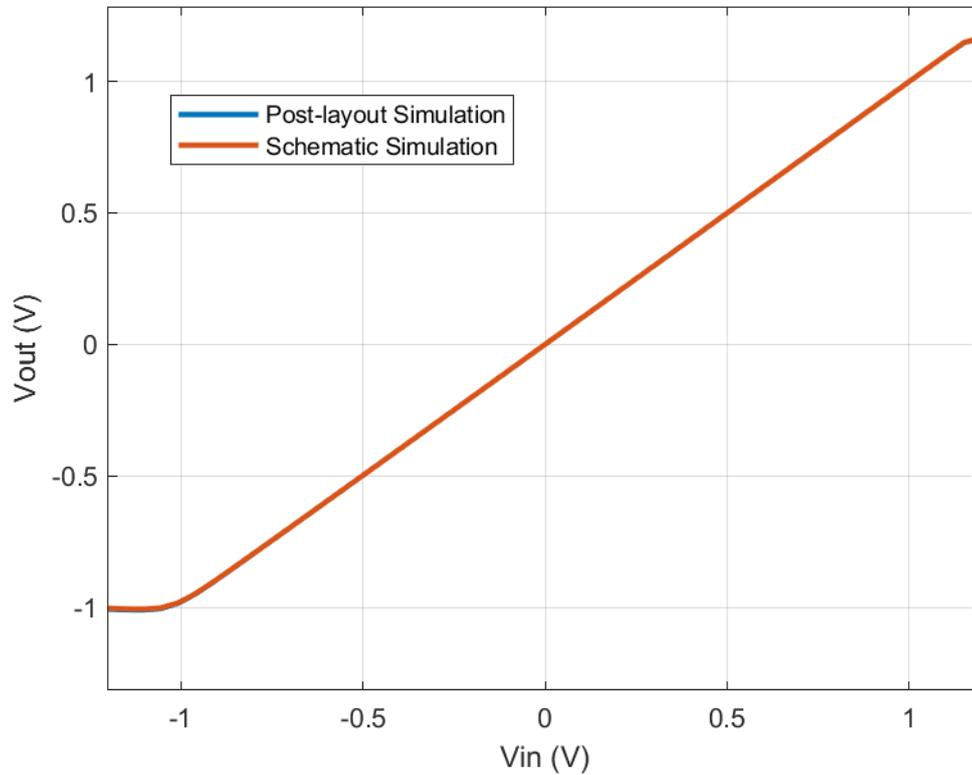
**Figure 3.14** – Schematic vs post-layout of voltage output range
