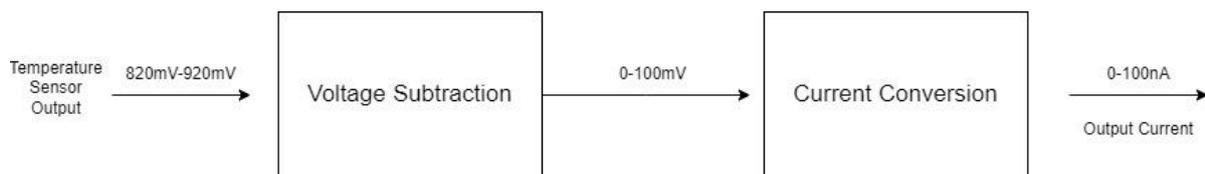
**Figure 3.1** – VI converter block diagram
