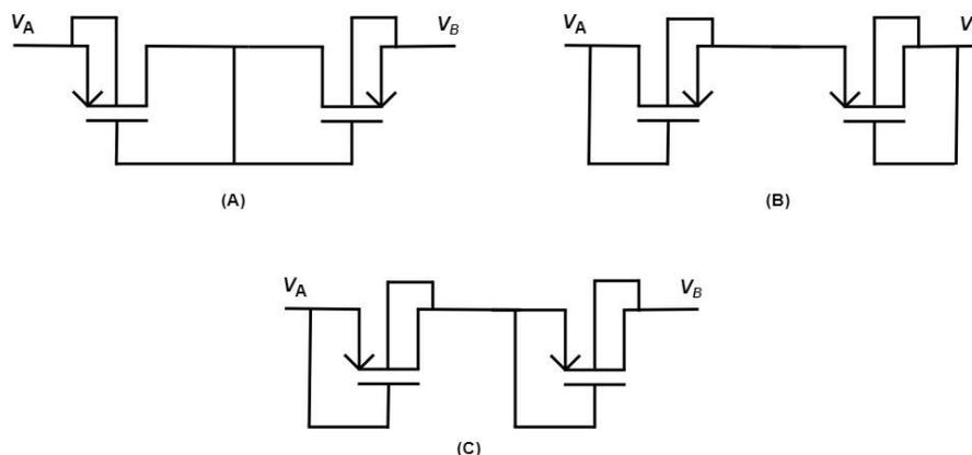
**Figure 2.20** – Multi-cell non-tuneable pseudo-resistor structure: (a) Two series connected PMOS transistors in gate-drain connected diode configuration and source-connected bulks; (b) two series-connected PMOS transistors with a common source and gate-drain diode connection; (c) two regular series connected PMOS transistors
