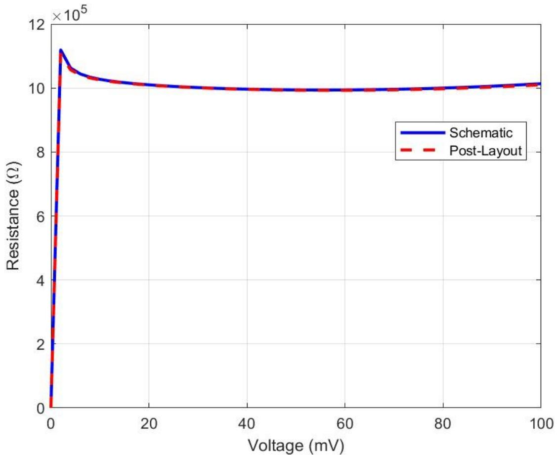
**Figure 4.16** – Resistance over input range for schematic and post-layout
