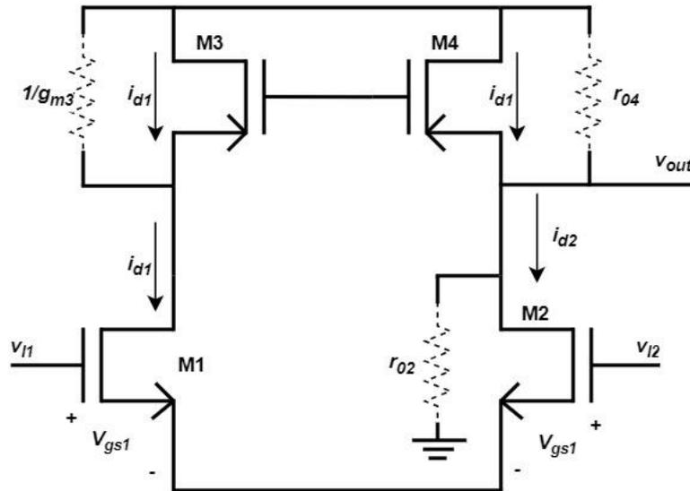
**Figure 2.13** – Small Signal model of single stage differential amplifier with active current mirror load
