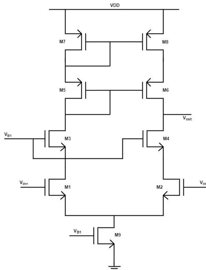
**Figure 2.17** – Telescopic OTA schematic
