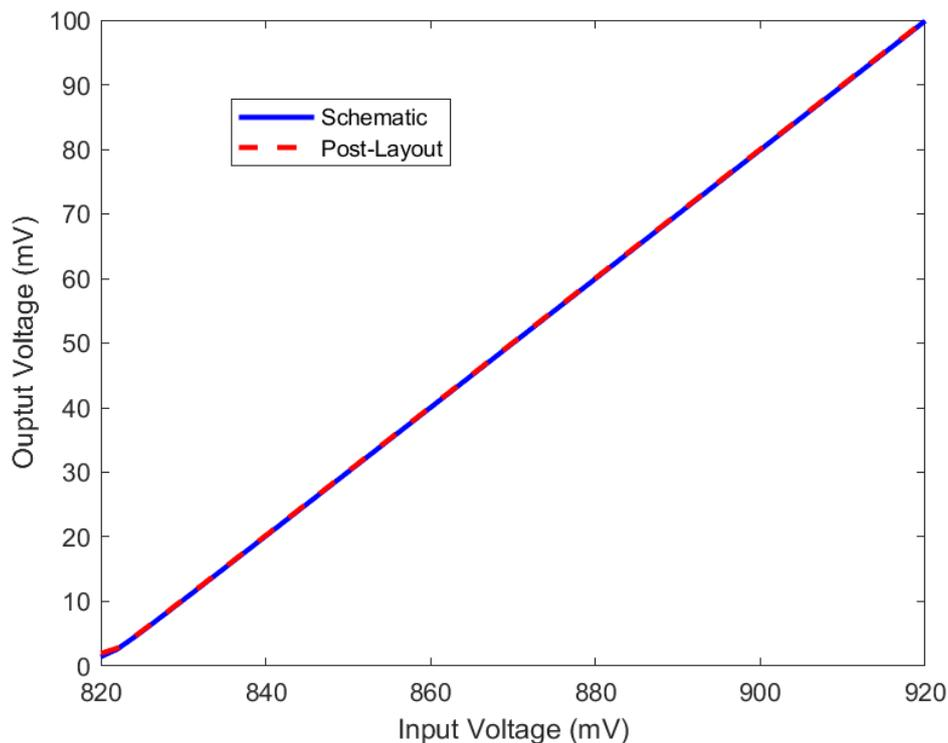
**Figure 5.6** – Schematic vs post layout voltage subtractor output
