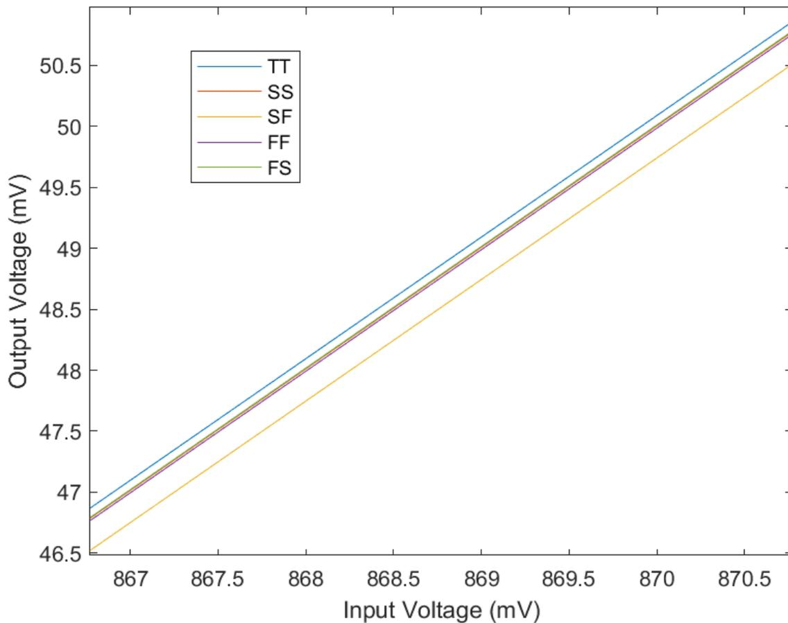
**Figure 5.4** – Zoomed in plot of subtracted voltage tested against the process corners
