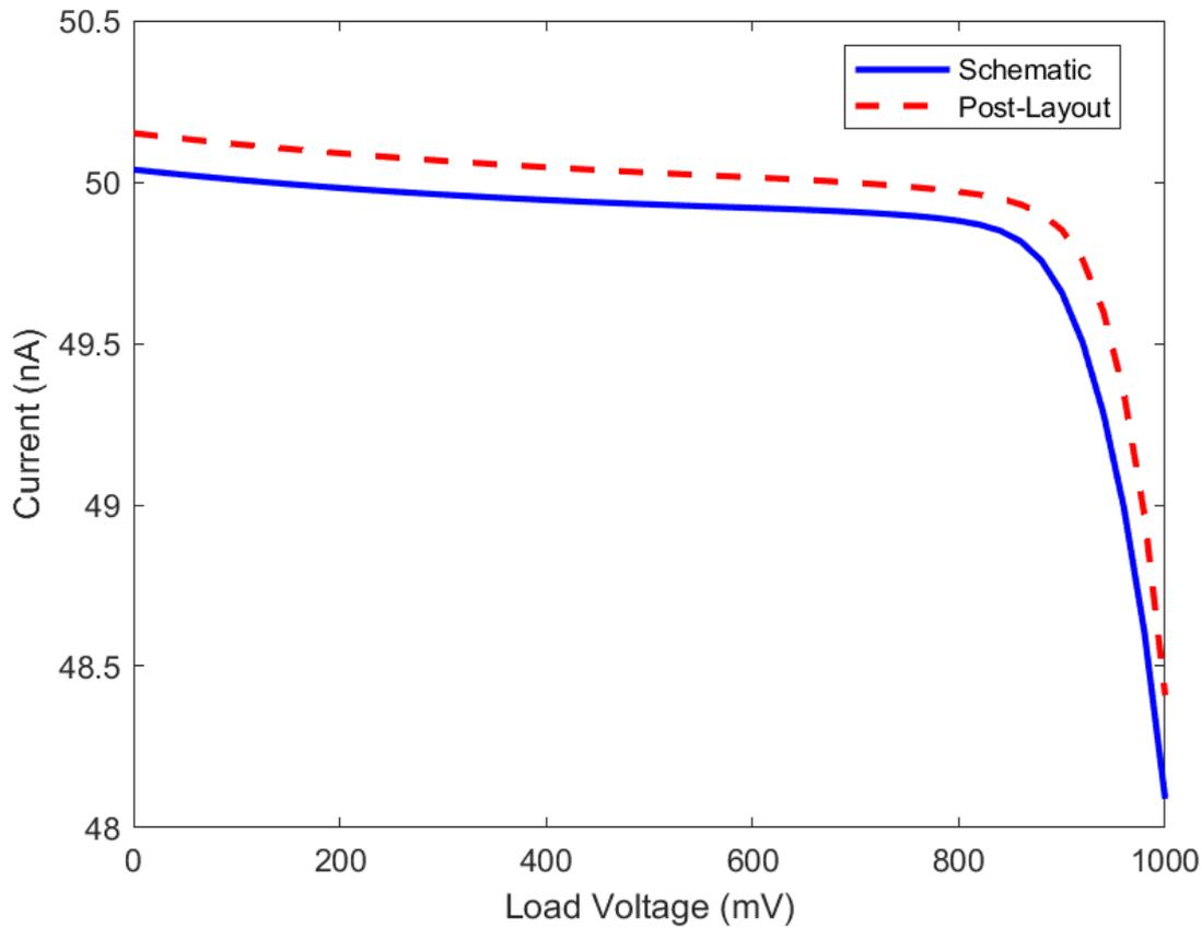
**Figure 5.15** – Output current with varied load voltage
