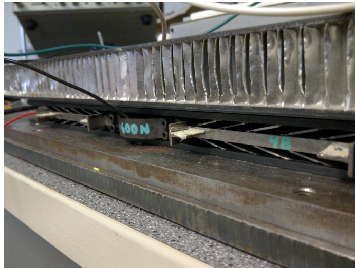
Fig. 3.2 Mechanical amplifier of piezoelectric actuator shown as described by Gustavsson's patent in [1]
