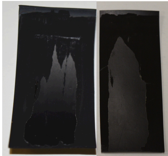
Figure 17: Samples showing the progression in top finish delamination. As the peel test continues, the delaminating area steadily increases, limited by the full width of the adhesion test tape.
